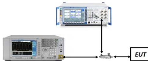
Figure 7-4. Test Instrument & Measurement Setup
