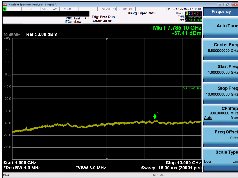
Plot 7-15. Conducted Spurious Plot (CDMA - Ch. 476)
