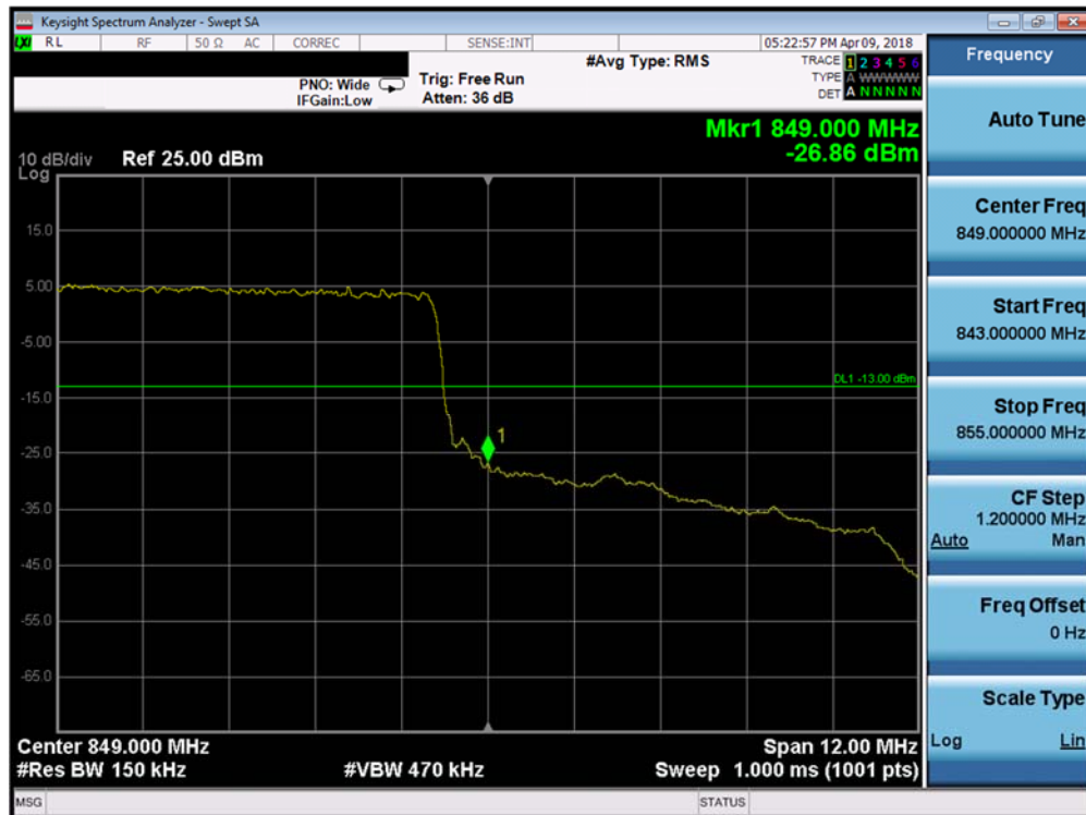
Plot 7-148. Upper Band Edge Plot (Band 26 - 15.0MHz QPSK - Full RB Configuration)
