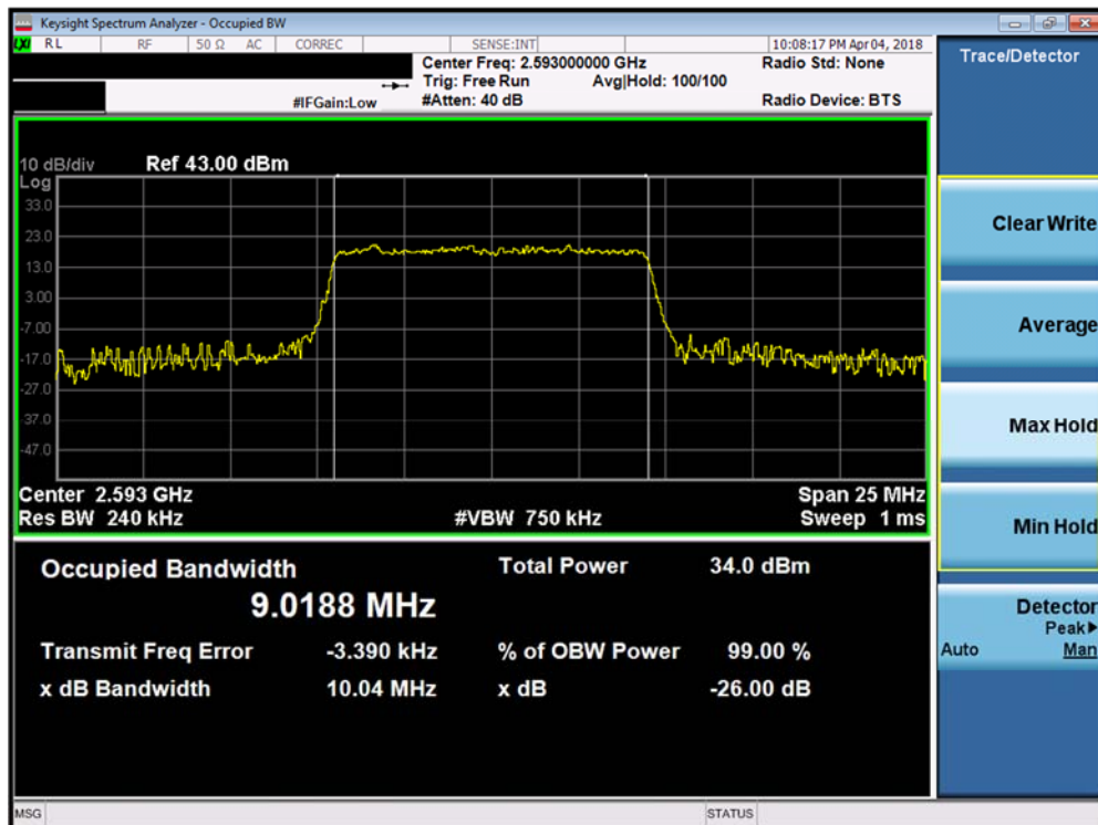
Plot 7-50. Occupied Bandwidth Plot (Band 41 PC2- 10.0MHz 16-QAM - Full RB Configuration)
