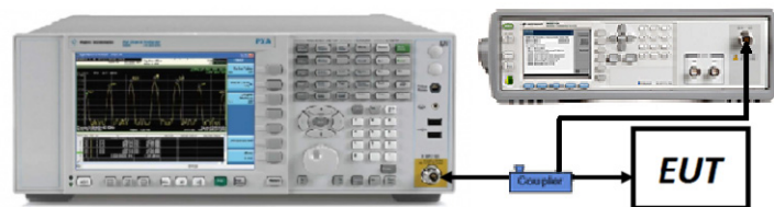
Figure 7-7. Test Instrument & Measurement Setup
