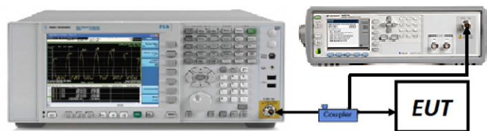
Figure 7-5. Test Instrument & Measurement Setup
