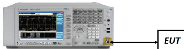
Figure 7-5. Test Instrument & Measurement Setup
