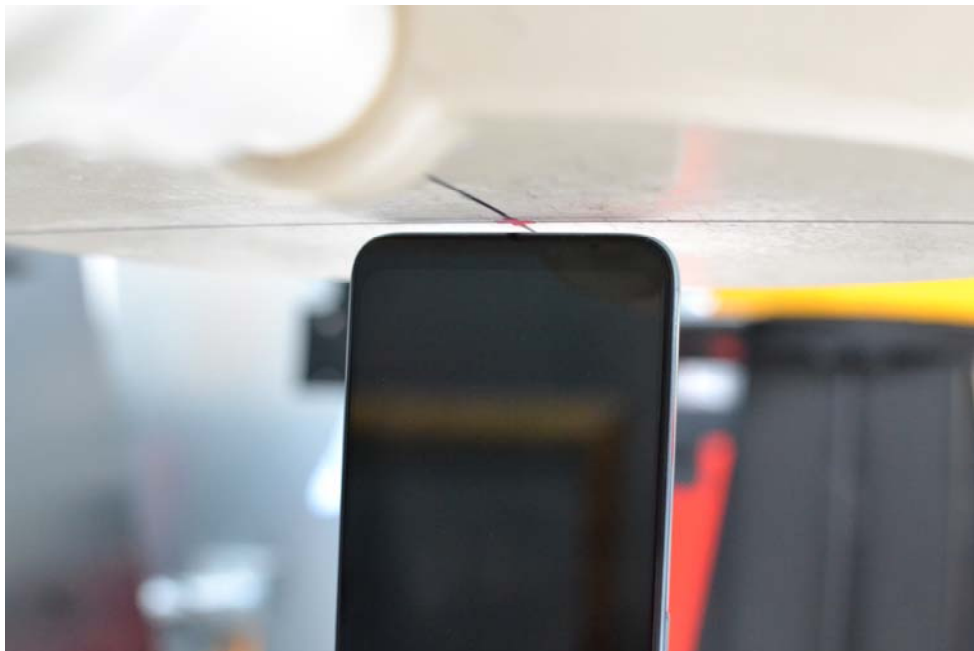
SAR Test Setup Photo 15: Bottom at 3 mm
