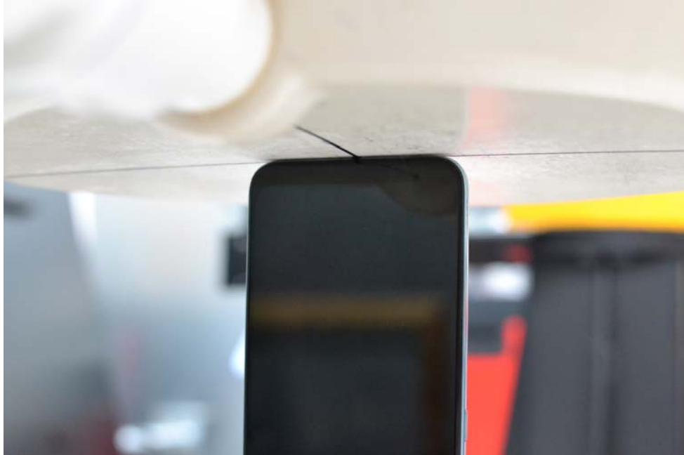
SAR Test Setup Photo 16: Bottom at 0 mm
