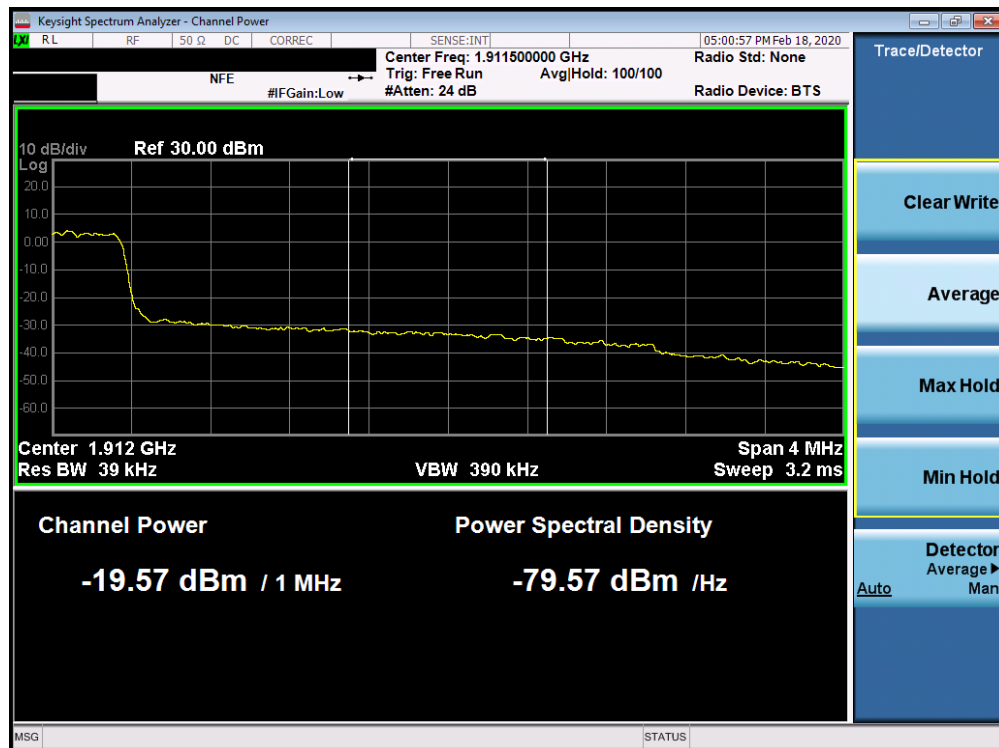
Plot 7-179. Upper Extended Band Edge Plot (Band 2 - 3.0MHz QPSK - Full RB Configuration)
