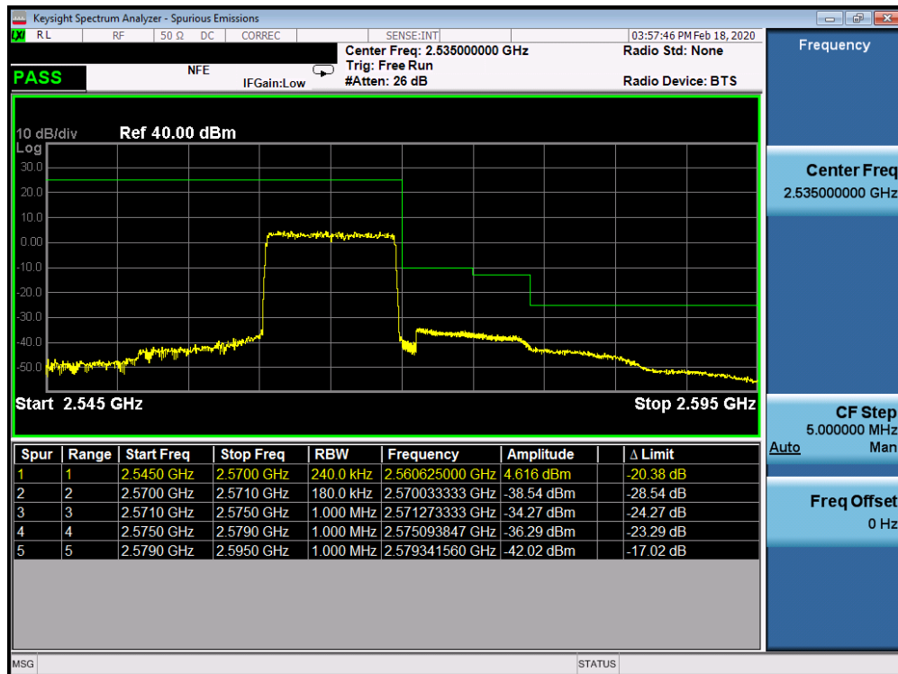
Plot 7-217. Higher ACP Plot (Band 7 - 10.0MHz QPSK - Full RB Configuration)
