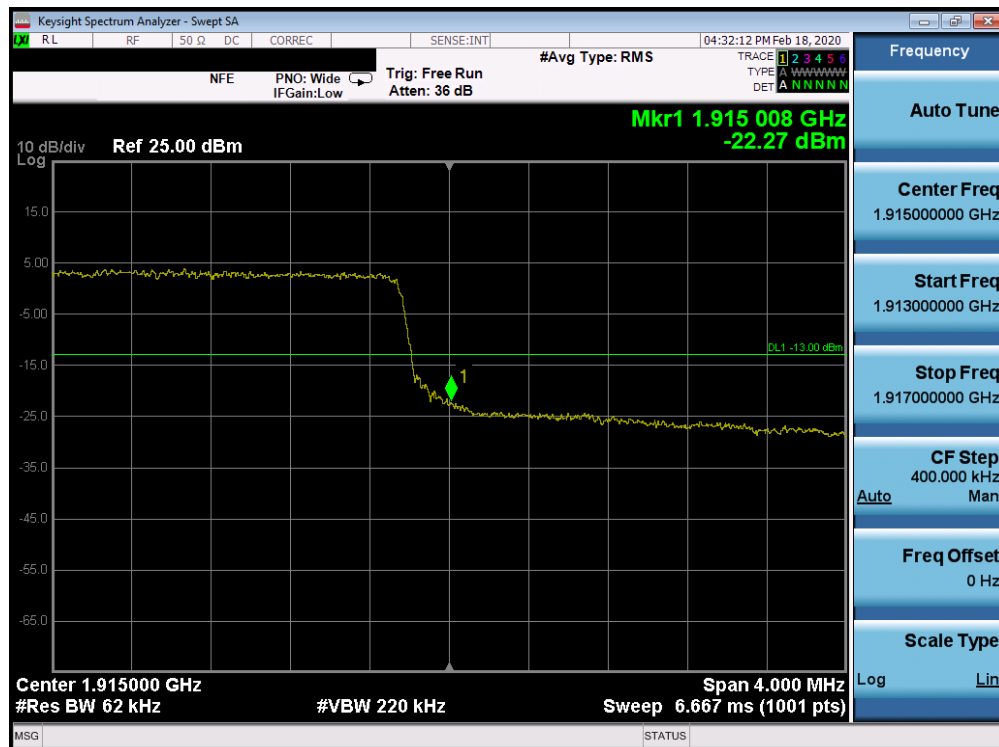
Plot 7-186. Upper Band Edge Plot (Band 25 - 5.0MHz QPSK - Full RB Configuration)
