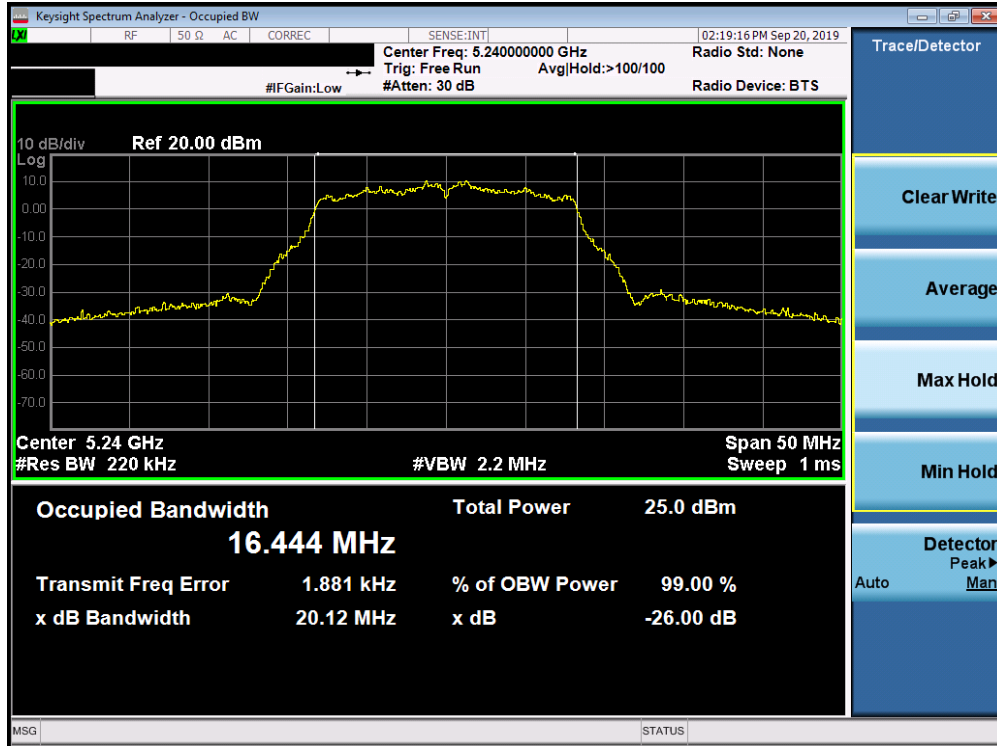
Plot 7-3. 26dB Bandwidth Plot (802.11a (UNII Band 1) – Ch. 48)
