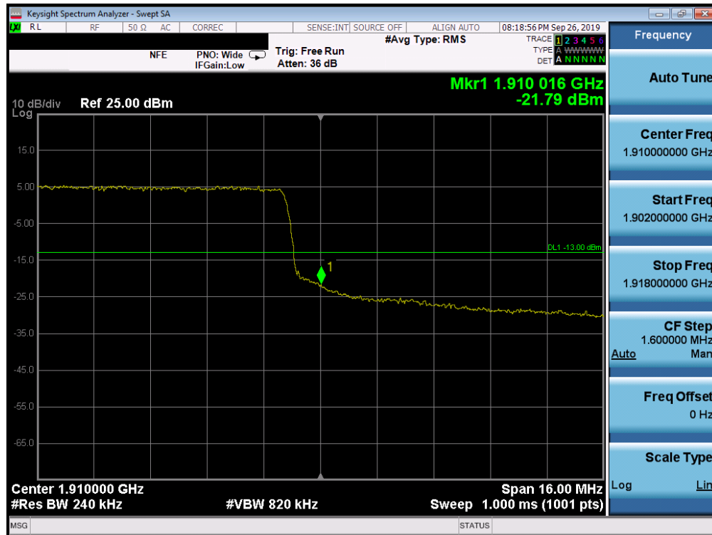
Plot 7-276. Upper Band Edge Plot (Band 2 - 20.0MHz QPSK - Full RB Configuration)
