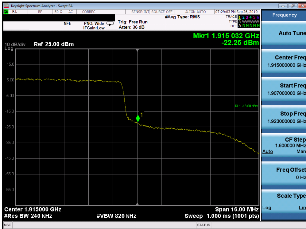
Plot 7-278. Upper Band Edge Plot (Band 25 - 20.0MHz QPSK - Full RB Configuration)
