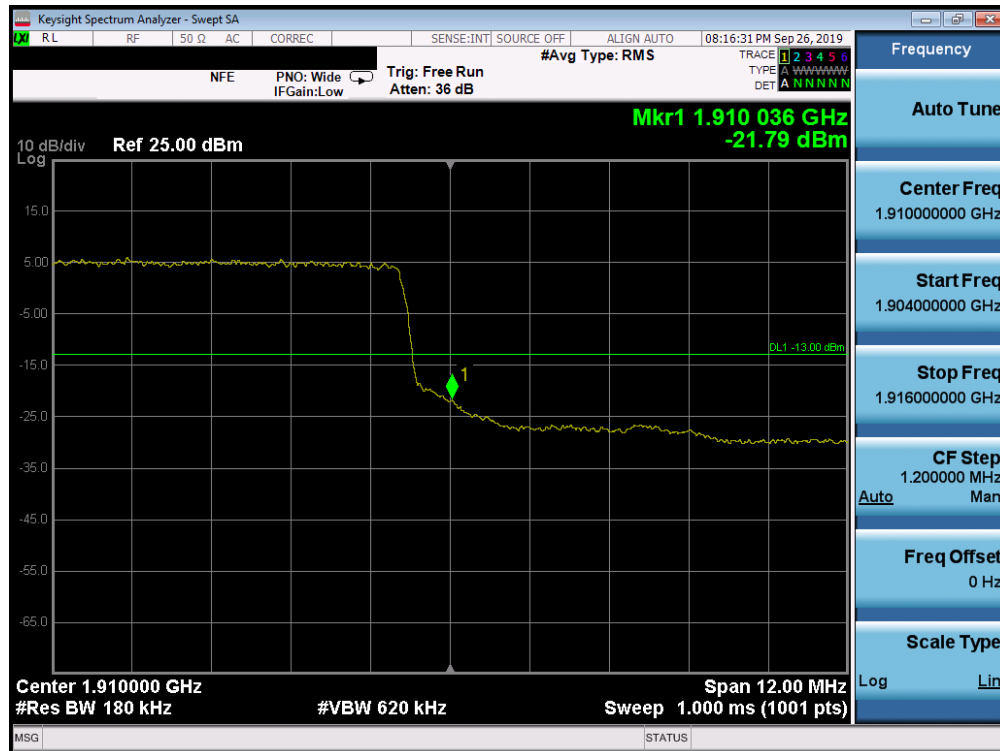
Plot 7-270. Upper Band Edge Plot (Band 2 - 15.0MHz QPSK - Full RB Configuration)
