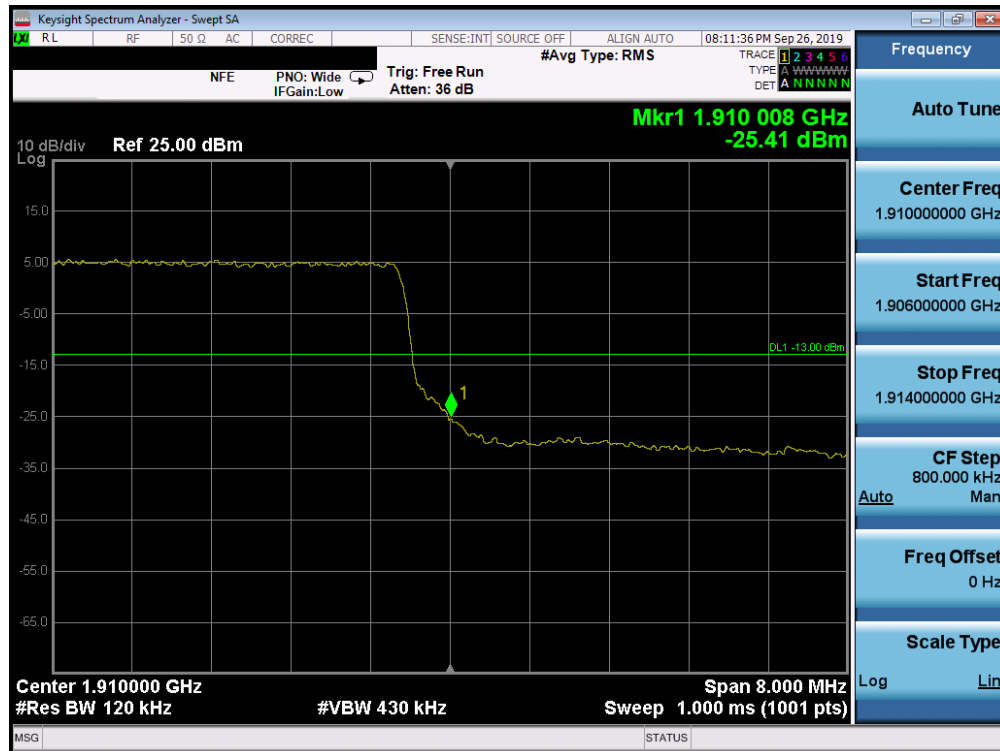
Plot 7-264. Upper Band Edge Plot (Band 2 - 10.0MHz QPSK - Full RB Configuration)
