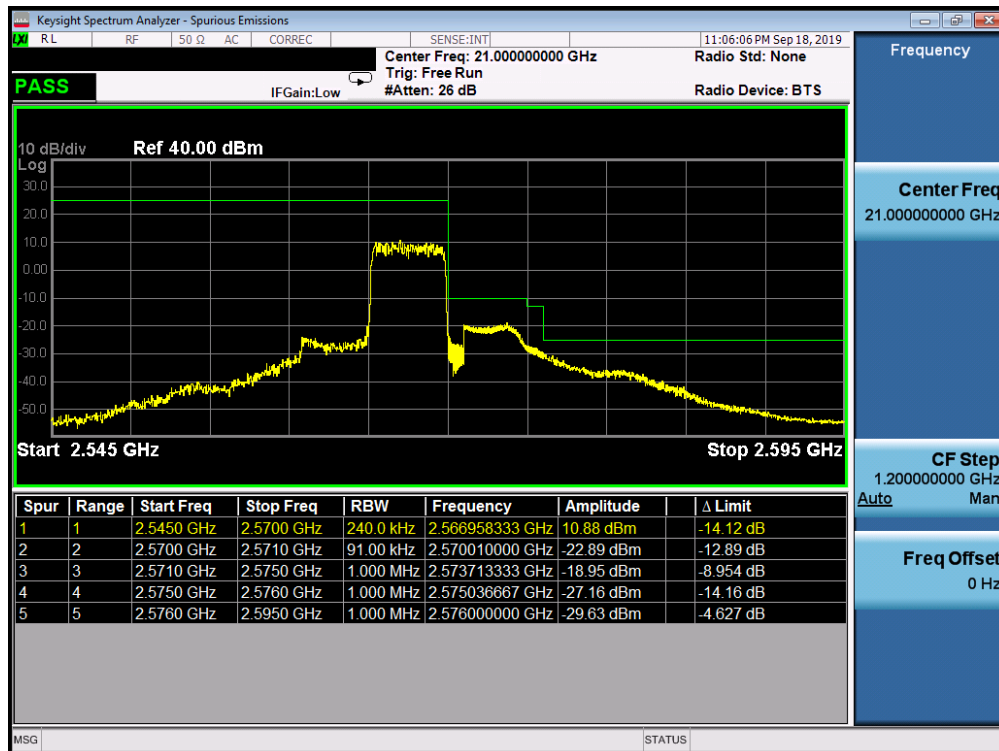
Plot 7-281. Upper ACP Plot (Band 7 - 5.0MHz QPSK - Full RB Configuration)
