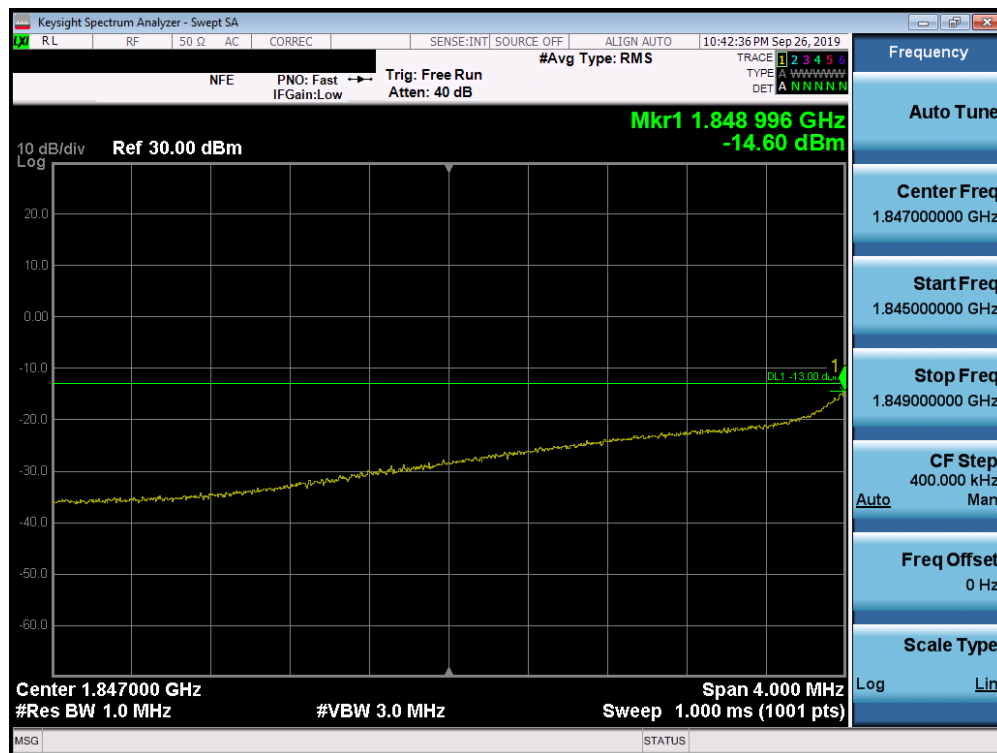
Plot 7-94. 4MHz Span Plot (PCS WCDMA Mode - Low Channel)
