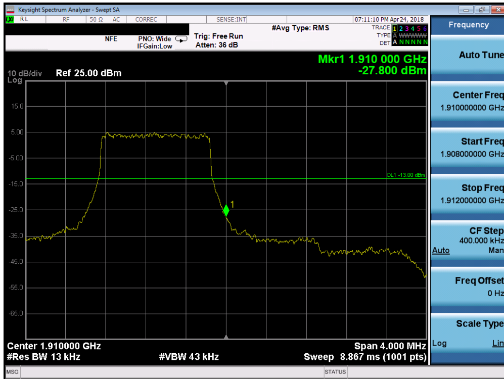
Plot 7-218. Upper Band Edge Plot (Band 2 - 1.4MHz QPSK - Full RB Configuration)
