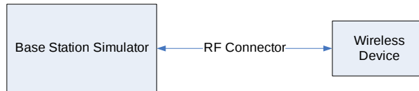
Figure 9-2 Power Measurement Setup
