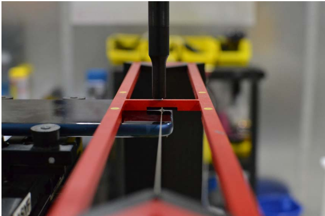
Figure 18-2 HAC Phantom Plane Alignment
