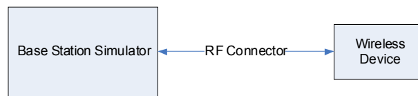
Figure 11-1 Power Measurement Setup
