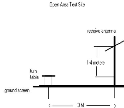
**Figure 3-1. Diagram of 3-meter outdoor test range**
