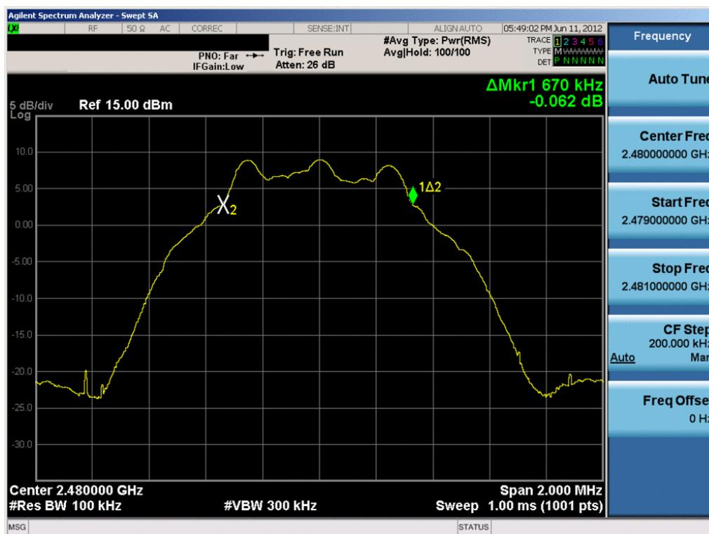
Plot 6-3. 6dB Bandwidth Plot (Bluetooth (LE) – Ch. 39)
