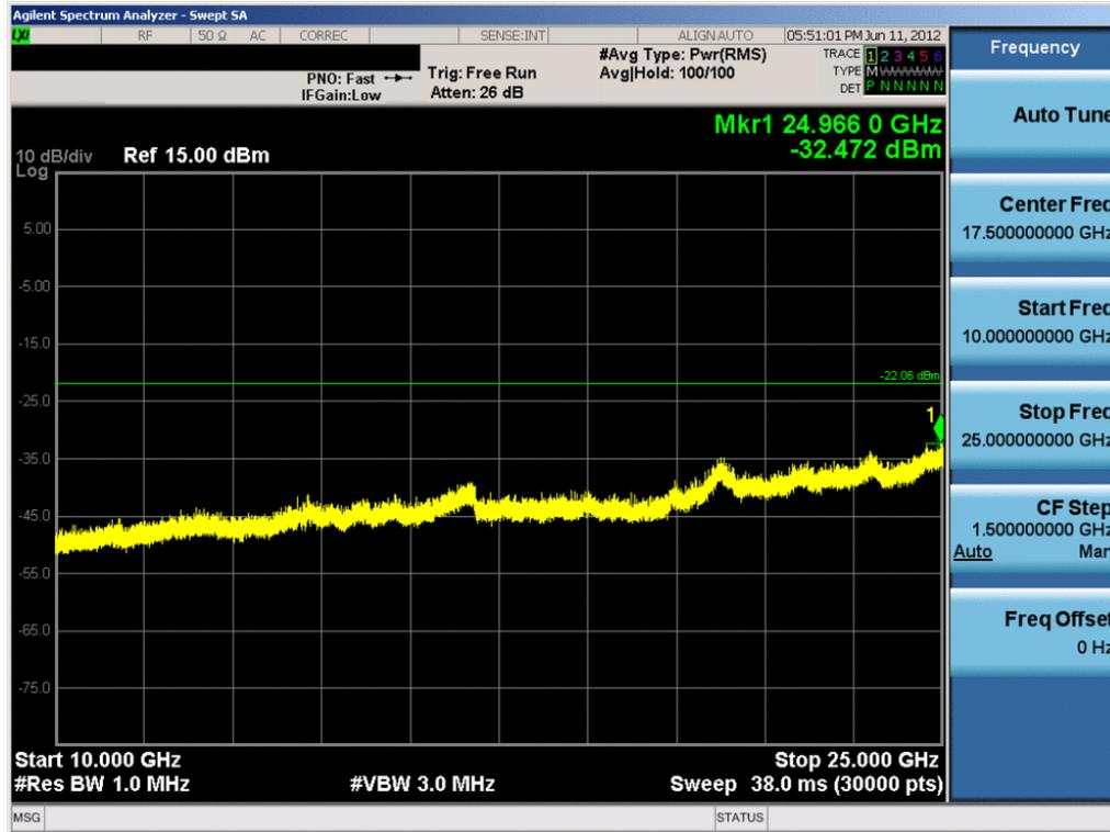
Plot 6-14. Conducted Spurious Plot (Bluetooth (LE) – Ch. 39)
