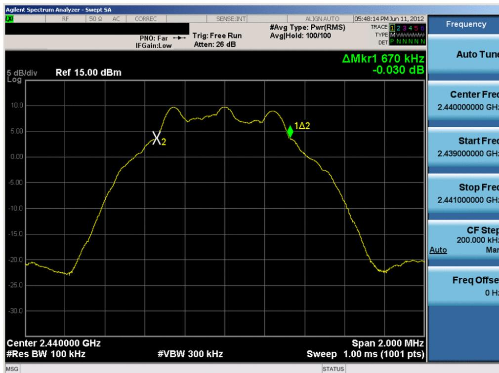
Plot 6-2. 6dB Bandwidth Plot (Bluetooth (LE) – Ch. 19)
