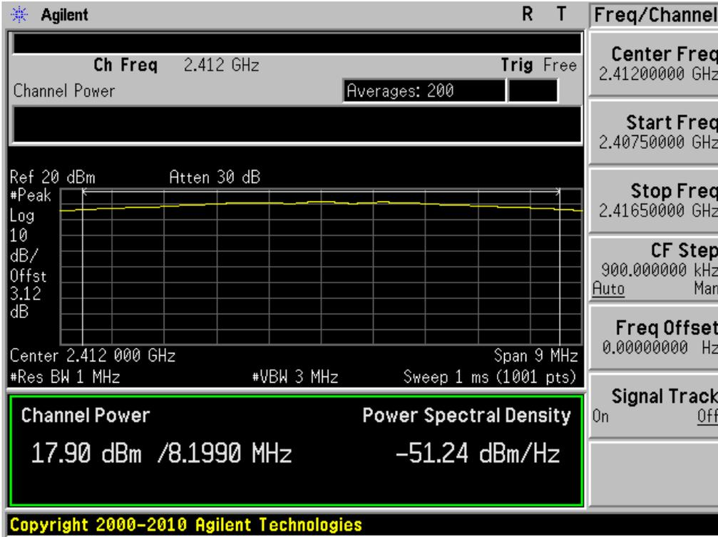
**Peak Output Power**      Test Mode: 802.11b & 1Mbps & 2437MHz
