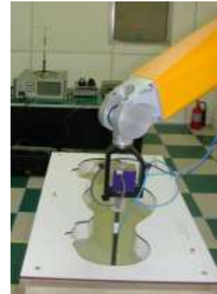
Figure 4.2 Photograph of the probe and the Phantom
