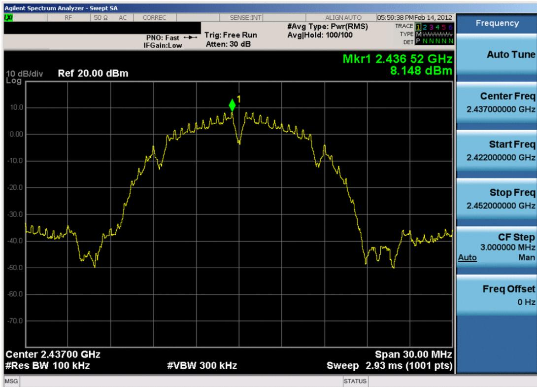
Plot 6-11. Power Spectral Density Plot (802.11b – Ch. 6)
