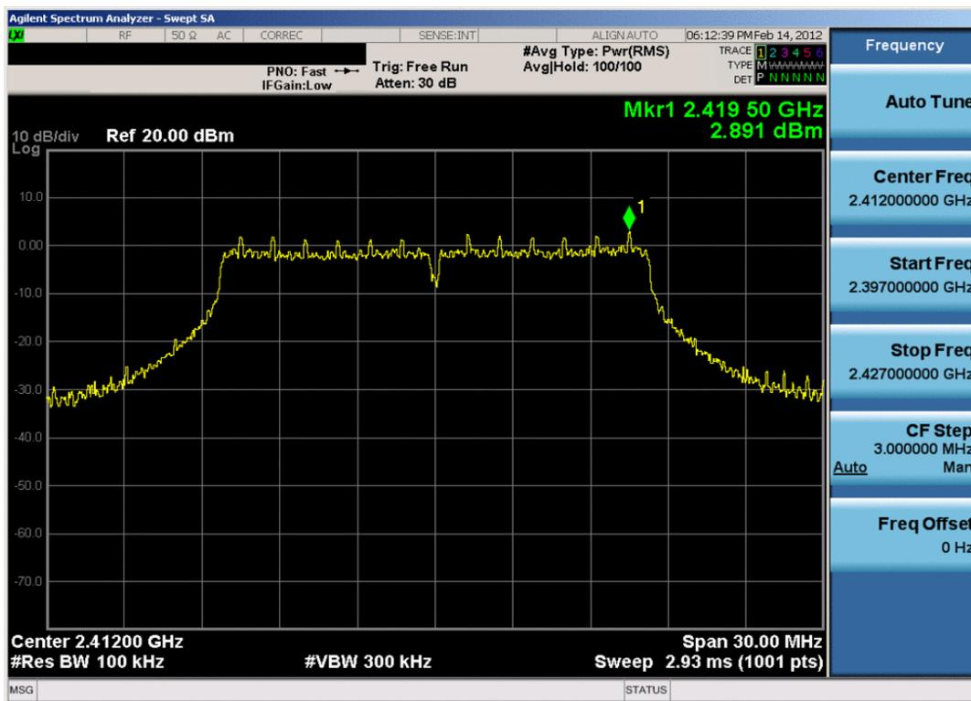
Plot 6-13. Power Spectral Density Plot (802.11g – Ch. 1)
