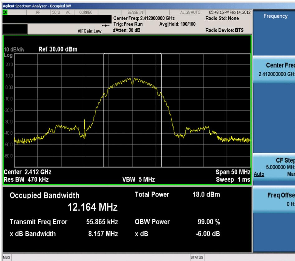
Plot 6-1. 6dB Bandwidth Plot (802.11b – Ch. 1)
