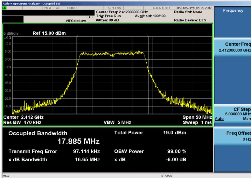
Plot 6-4. 6dB Bandwidth Plot (802.11g – Ch. 1)
