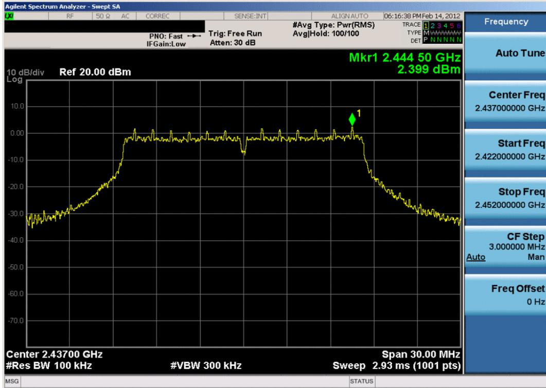
Plot 6-14. Power Spectral Density Plot (802.11g – Ch. 6)
