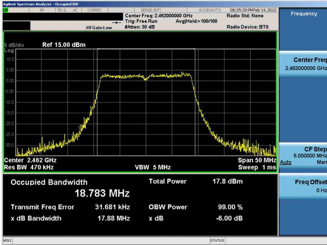
Plot 6-9. 6dB Bandwidth Plot (802.11n – Ch. 11)
