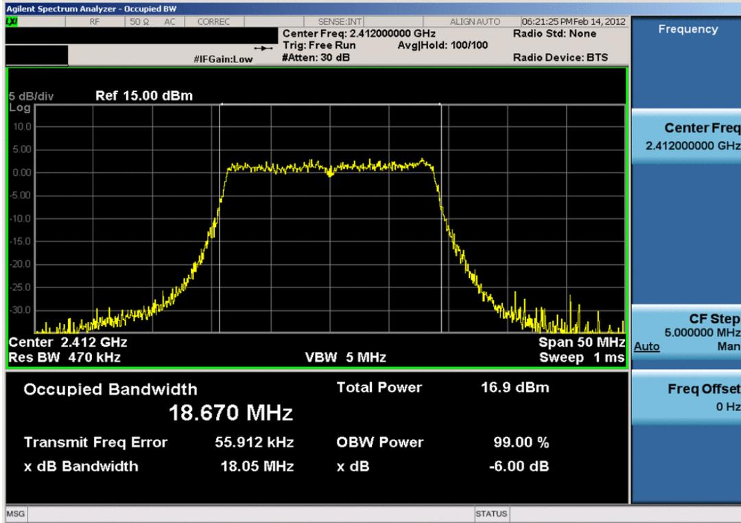
Plot 6-7. 6dB Bandwidth Plot (802.11n – Ch. 1)
