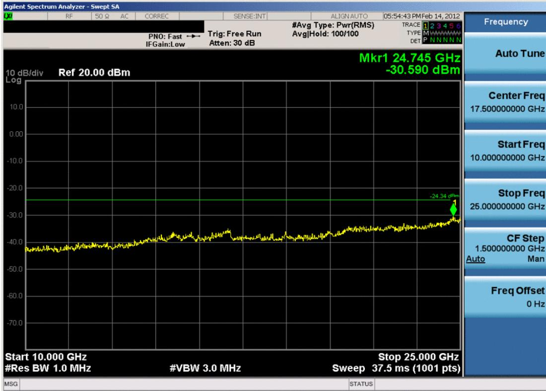
Plot 6-26. Conducted Spurious Plot (802.11b – Ch. 1)
