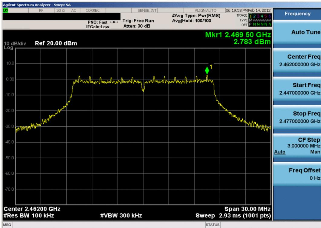
Plot 6-15. Power Spectral Density Plot (802.11g – Ch. 11)
