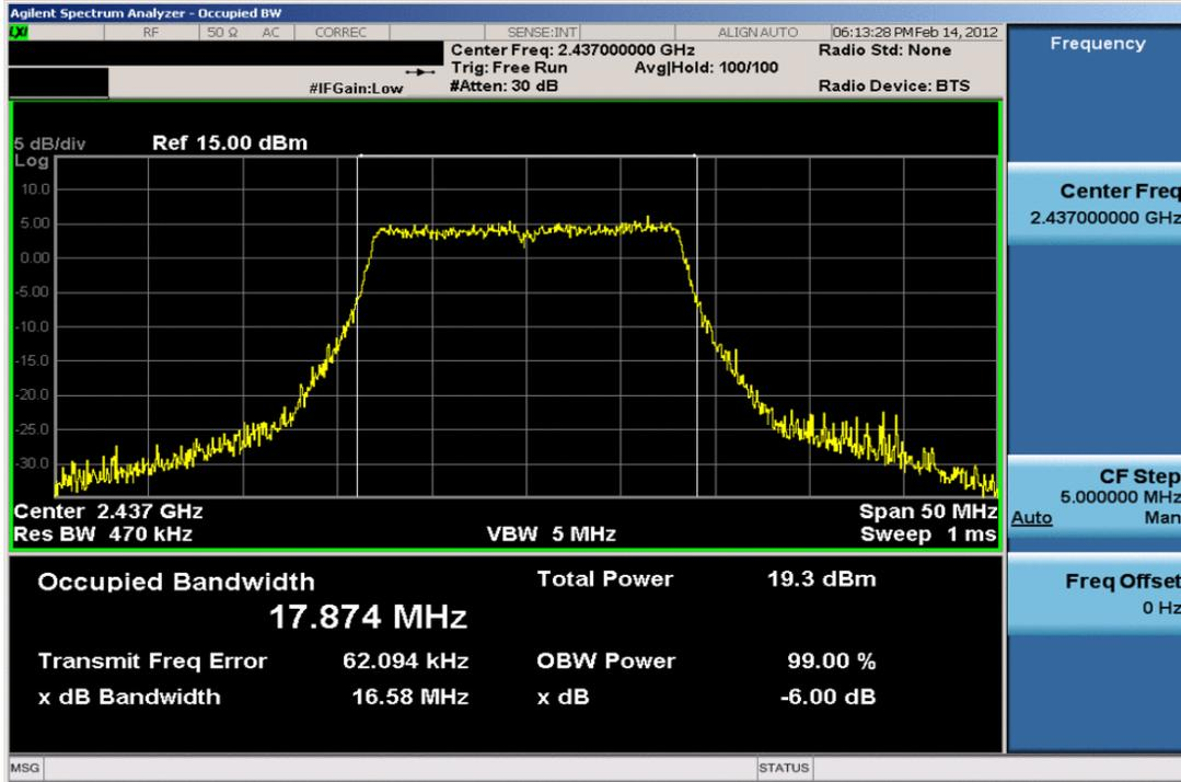
Plot 6-5. 6dB Bandwidth Plot (802.11g – Ch. 6)
