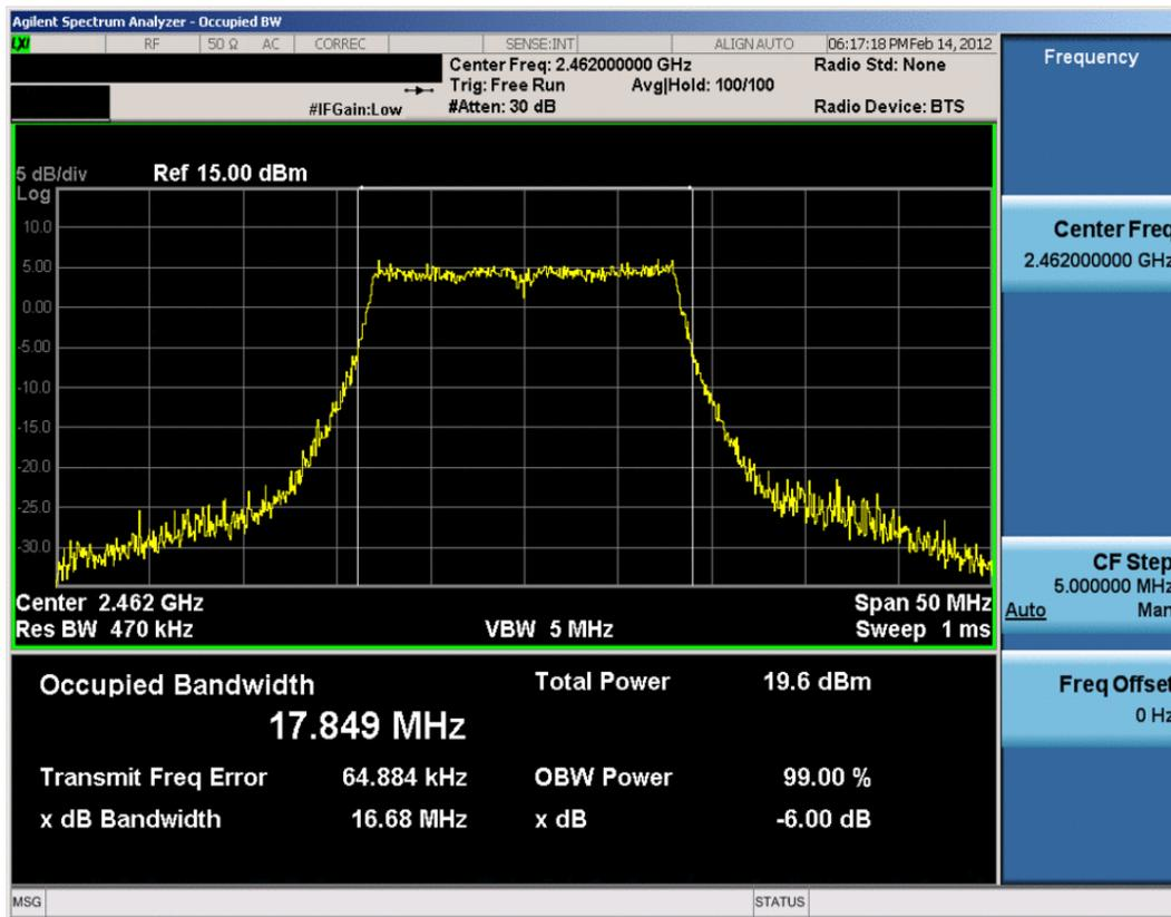
Plot 6-6. 6dB Bandwidth Plot (802.11g – Ch. 11)
