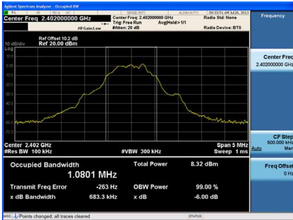
6dB Bandwidth plot (Low-CH 0)
