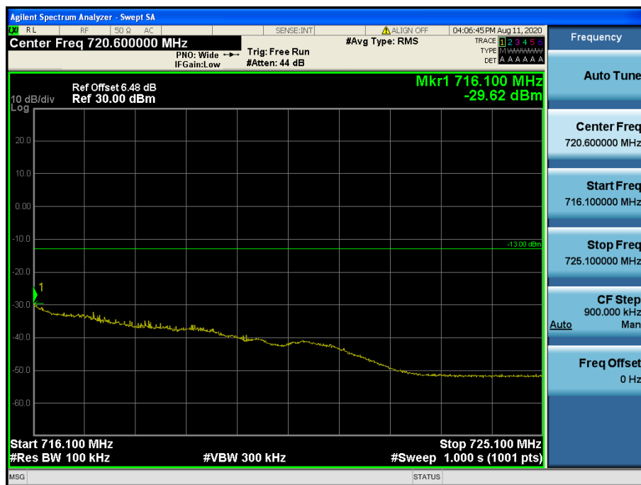
LTE Band 12 / 10 MHz / QPSK - RB Size/Offset (25/25)
