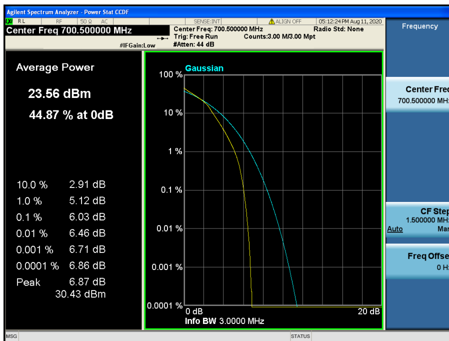
LTE Band 12 / 3 MHz / 16QAM - RB Size 15
