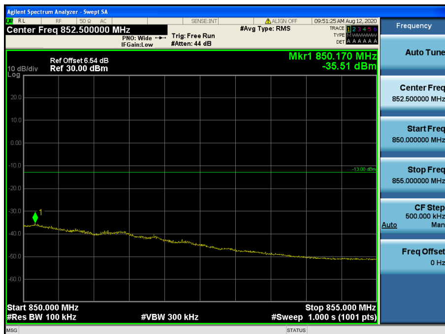
LTE Band 5 / 3 MHz / QPSK - RB Size/Offset (15/0)
