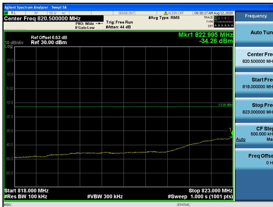
LTE Band 5 / 3 MHz / QPSK - RB Size/Offset (15/0)
