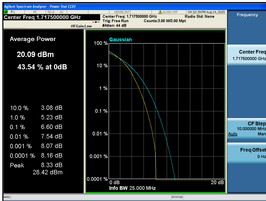
LTE Band 4 / 15 MHz / 64QAM - RB Size 75
