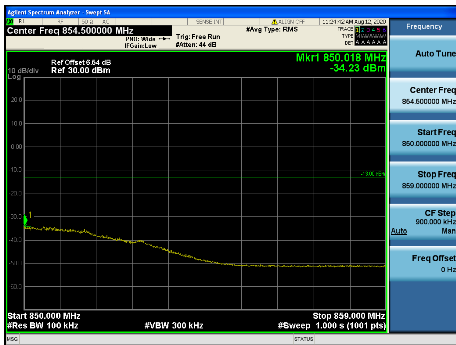
LTE Band 5 / 10 MHz / QPSK - RB Size/Offset (50/0)
