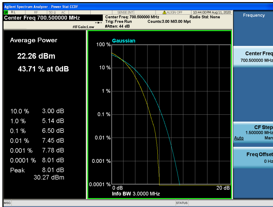
LTE Band 12 / 3 MHz / 64QAM - RB Size 15
