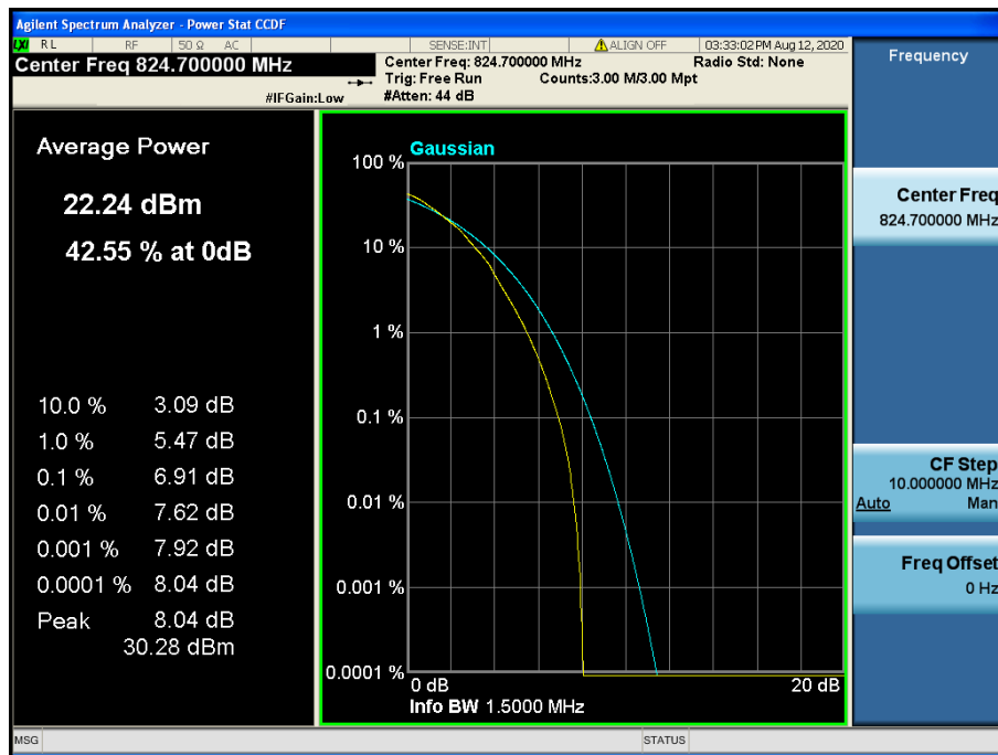
LTE Band 5 / 1.4 MHz / 64QAM - RB Size 6
