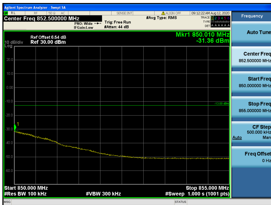
LTE Band 5 / 1.4 MHz / QPSK - RB Size/Offset (6/0)
