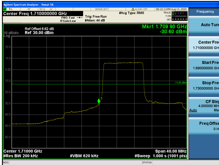
LTE Band 4 / 20 MHz / QPSK - RB Size/Offset (50/0)
