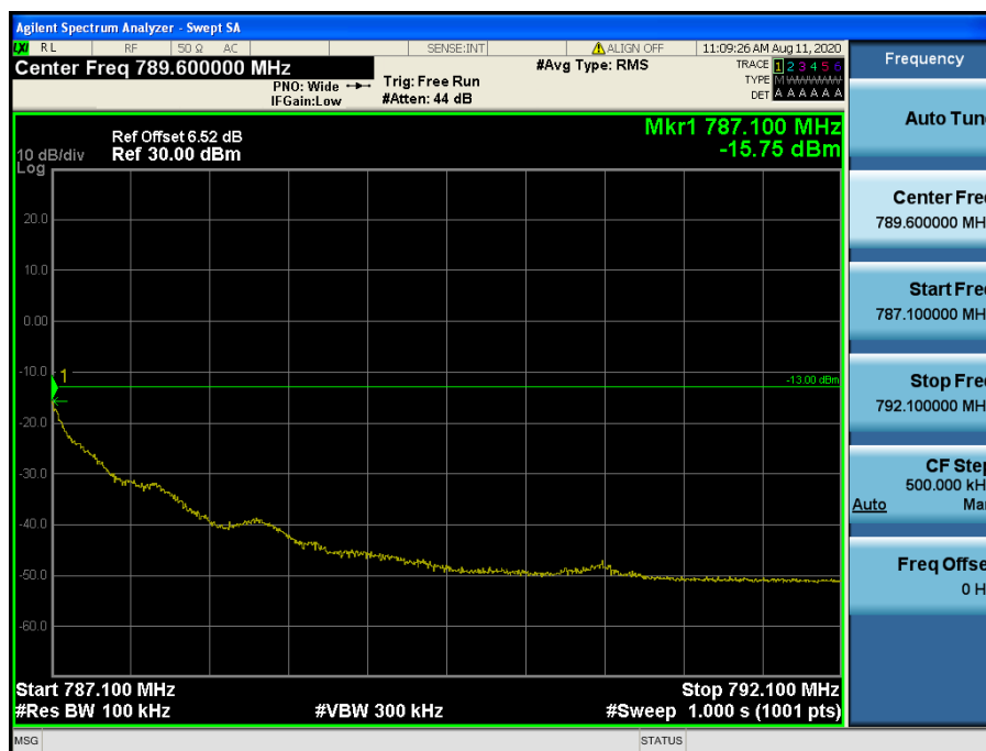
LTE Band 13 / 5 MHz / 16QAM - RB Size/Offset (1/24)
