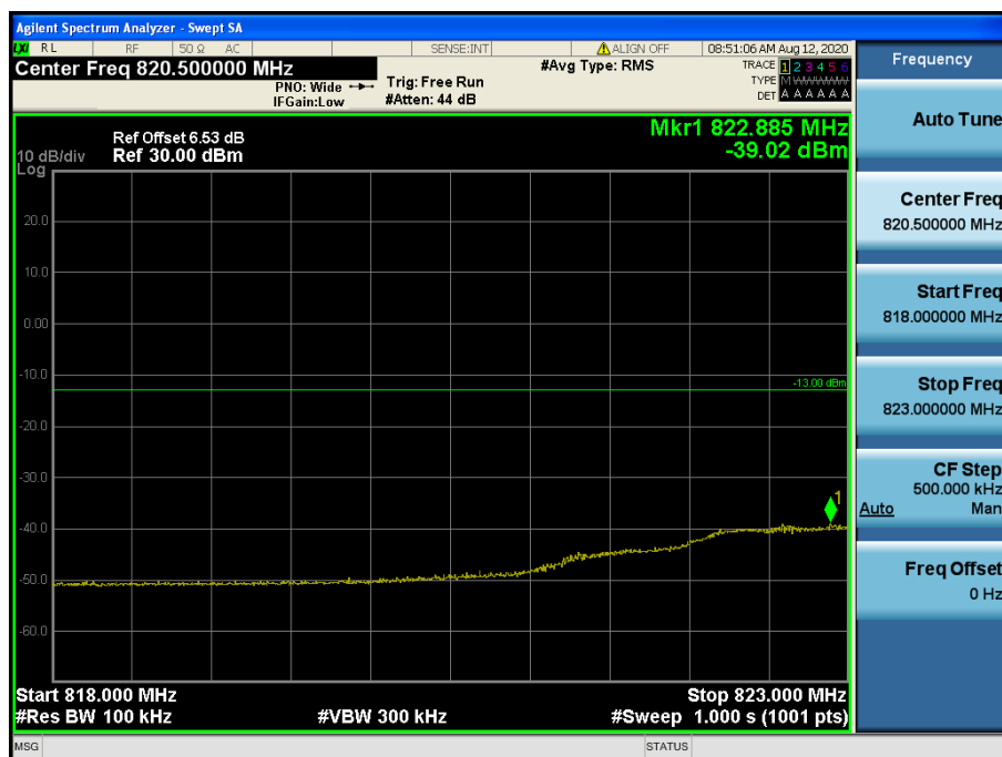
LTE Band 5 / 1.4 MHz / QPSK - RB Size/Offset (6/0)
