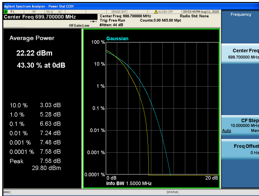
LTE Band 12 / 1.4 MHz / 64QAM - RB Size 6
