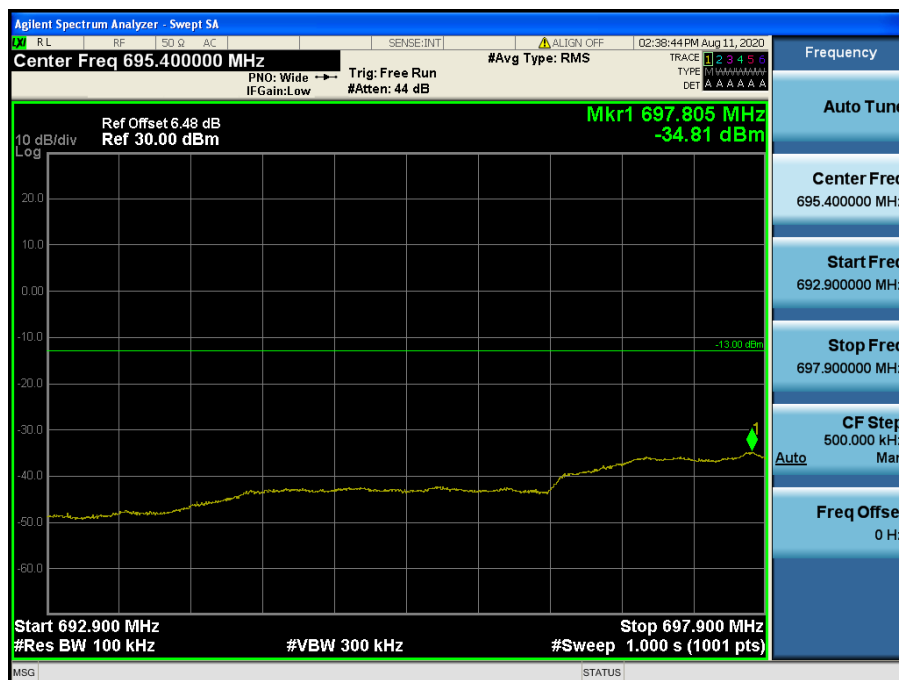
LTE Band 12 / 3 MHz / QPSK - RB Size/Offset (15/0)
