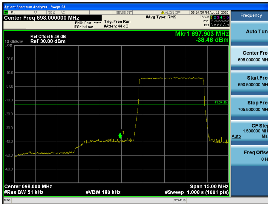
LTE Band 12 / 5 MHz / QPSK - RB Size/Offset (25/0)
