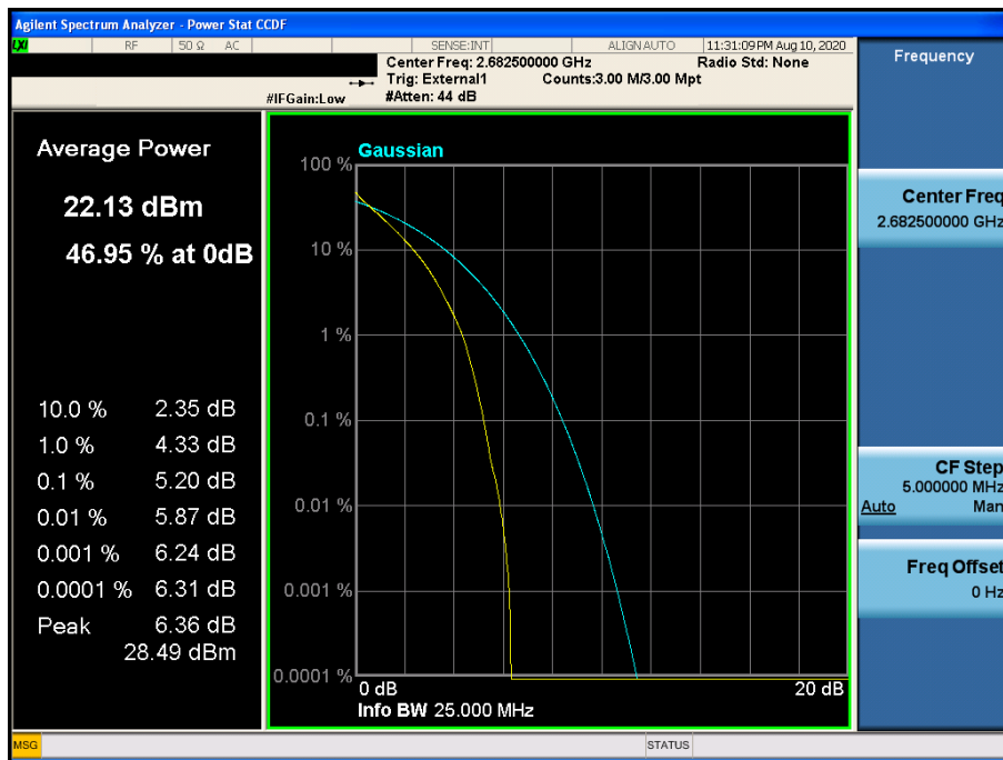
LTE Band 41 / 15 MHz / QPSK - RB Size 75
