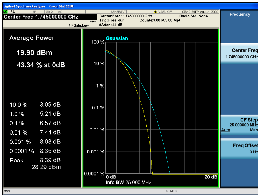
LTE Band 4 / 20 MHz / 64QAM - RB Size 100
