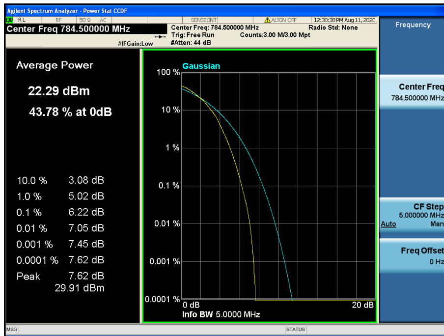
LTE Band 13 / 5 MHz / 64QAM - RB Size 25
