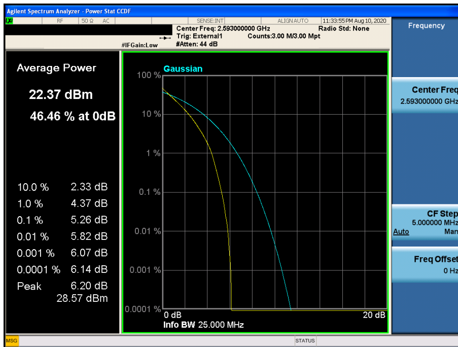
LTE Band 41 / 20 MHz / QPSK - RB Size 100
