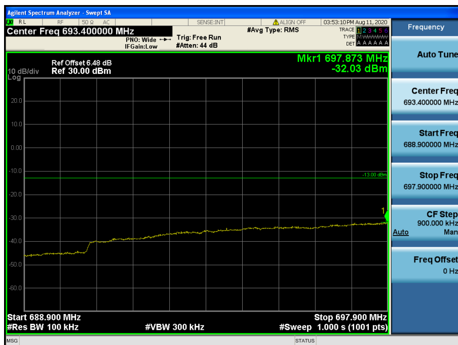
LTE Band 12 / 10 MHz / QPSK - RB Size/Offset (50/0)
