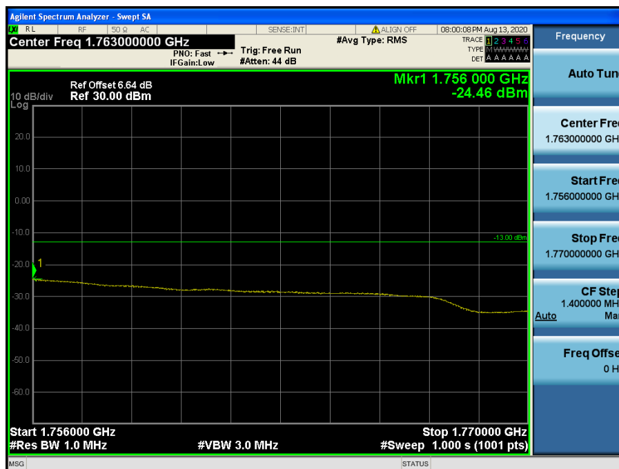
LTE Band 4 / 15 MHz / QPSK - RB Size/Offset (75/0)
