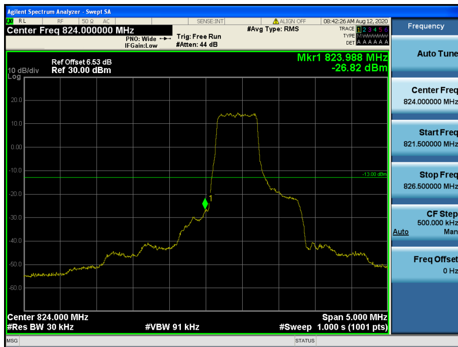
LTE Band 5 / 1.4 MHz / QPSK - RB Size/Offset (3/0)
