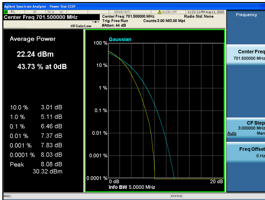
LTE Band 12 / 5 MHz / 64QAM - RB Size 25
