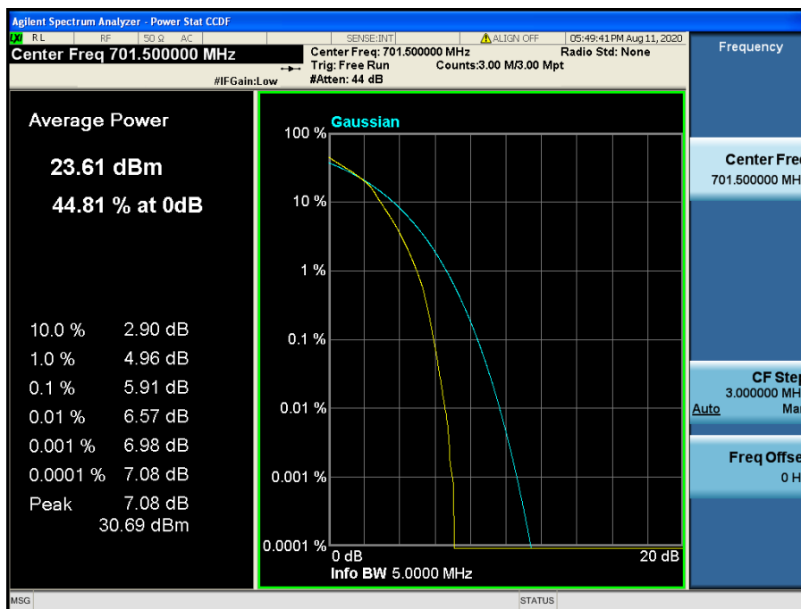
LTE Band 12 / 5 MHz / 16QAM - RB Size 25
