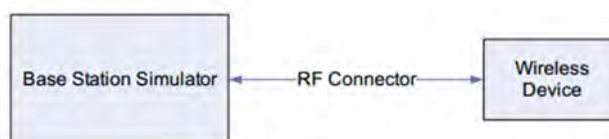
Figure 9.1 Power Measurement Setup
