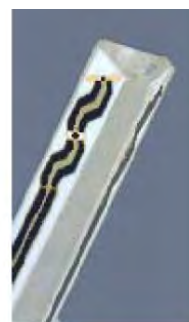
Figure E.2.2 Probe Thick-Film Technique
