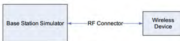
Figure 9.1 Power Measurement Setup
