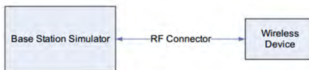
Figure 9.1 Power Measurement Setup
