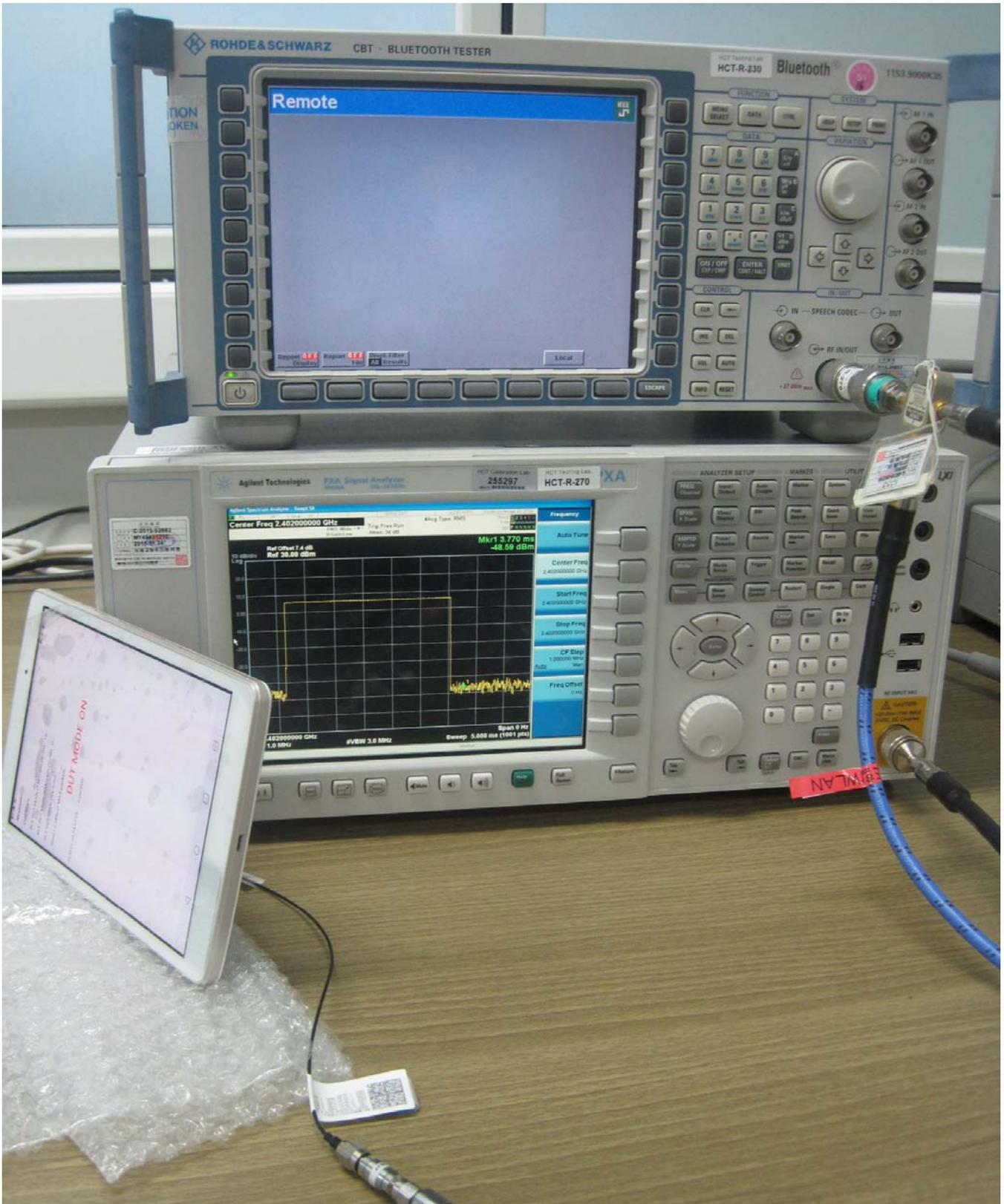
■ Conducted WLAN Test Setup Photo
