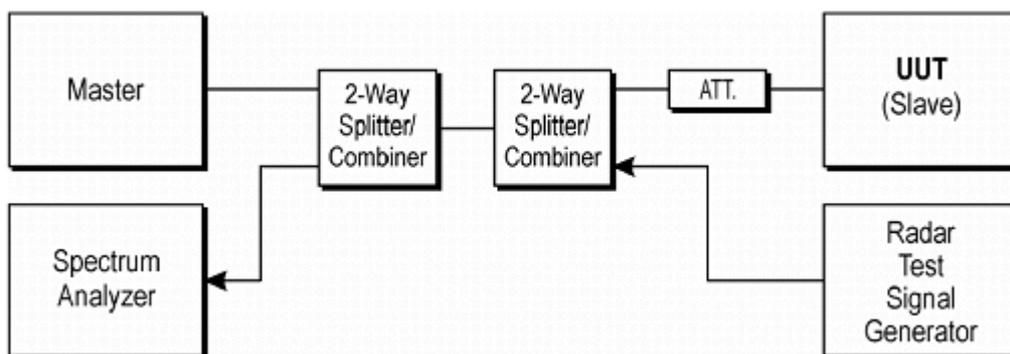
Figure 3-1. Conducted Test Setup for DFS
