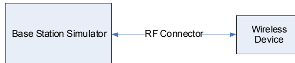
Figure 10-4 Power Measurement Setup
