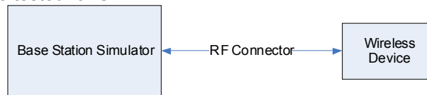
Figure 11-3 Power Measurement Setup
