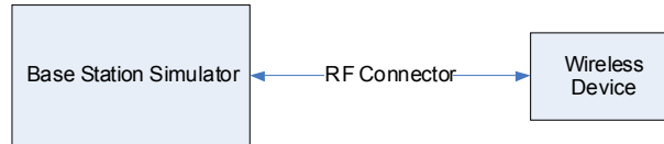
Figure 11-2 Power Measurement Setup
