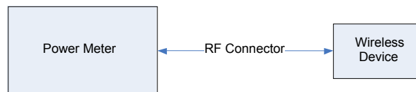
Figure 10-5 Power Measurement Setup
