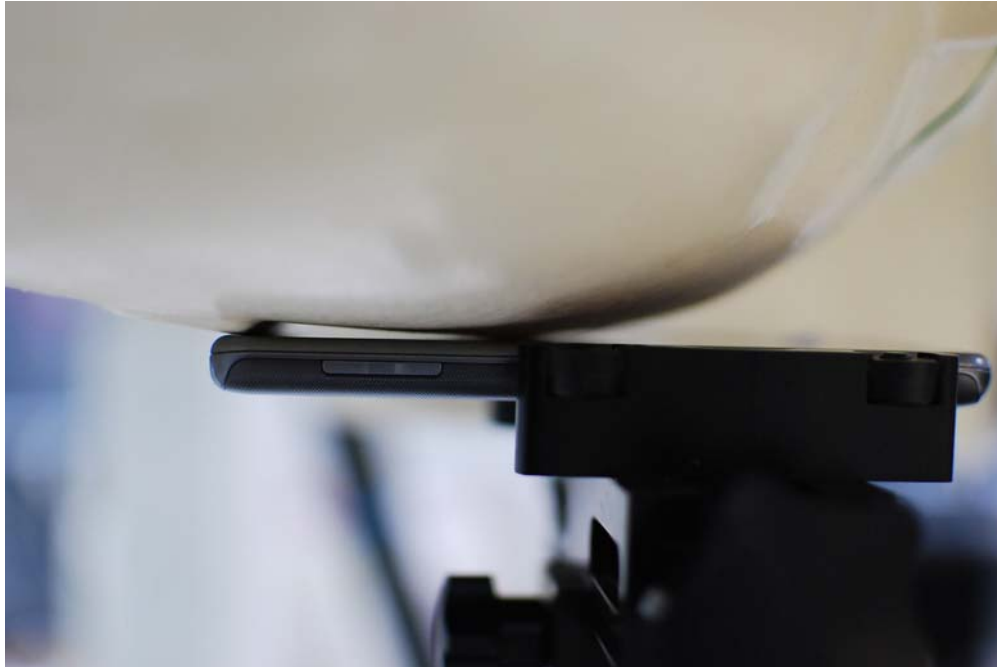
SAR Test Setup Photo 1 – Right Cheek
