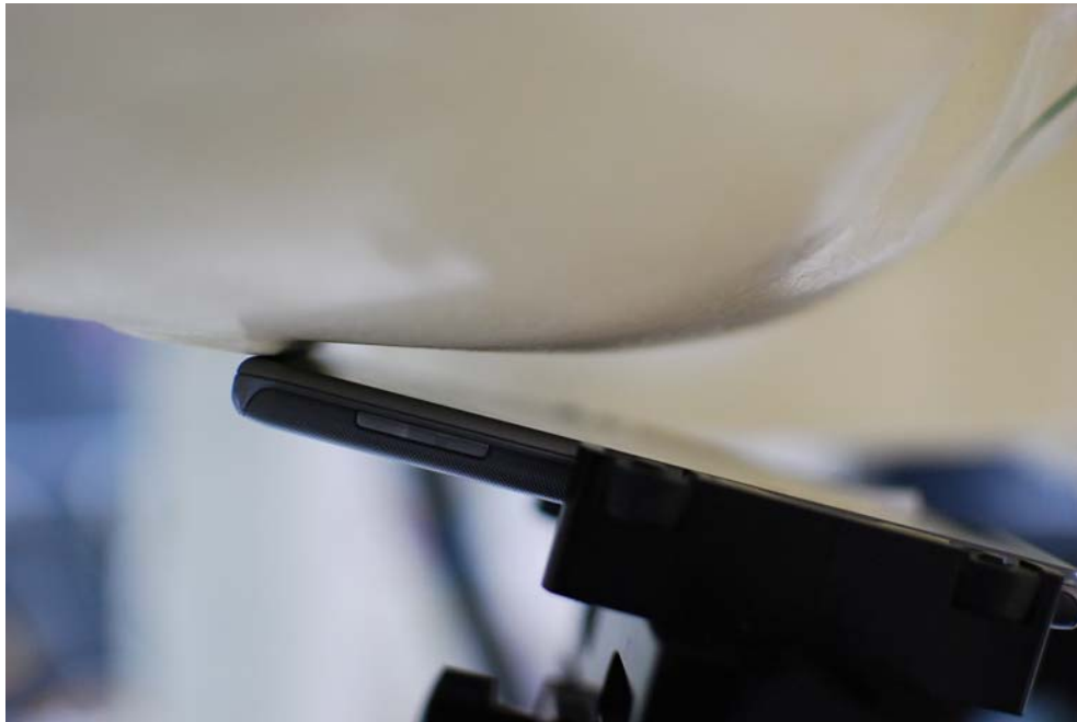
SAR Test Setup Photo 2 – Right Tilt
