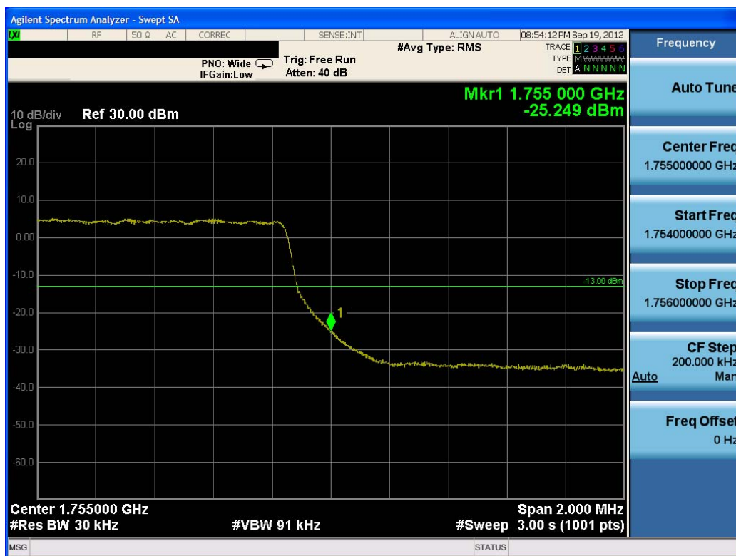
Plot 8-13. Upper Band Edge Plot (QPSK – RB Size 15)
