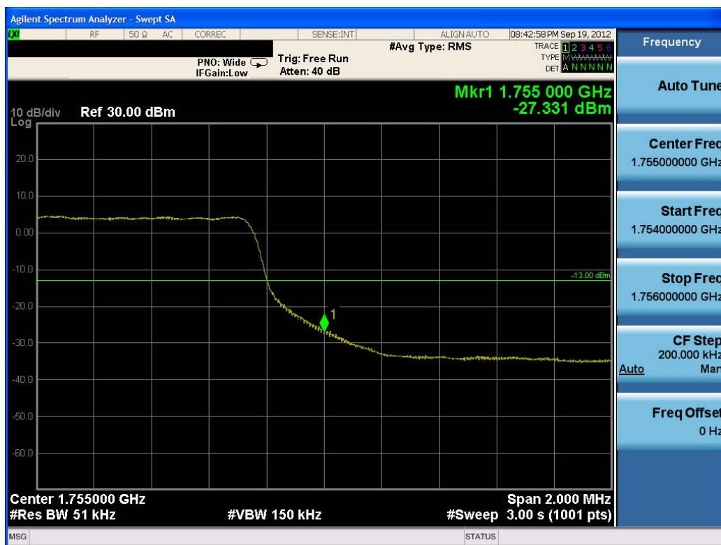
Plot 9-13. Upper Band Edge Plot (QPSK – RB Size 25)
