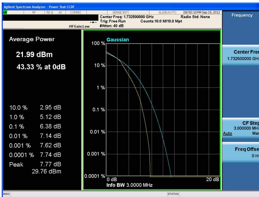
Plot 8-6. Peak to Average Ratio Plot (16QAM - RB Size 15)
