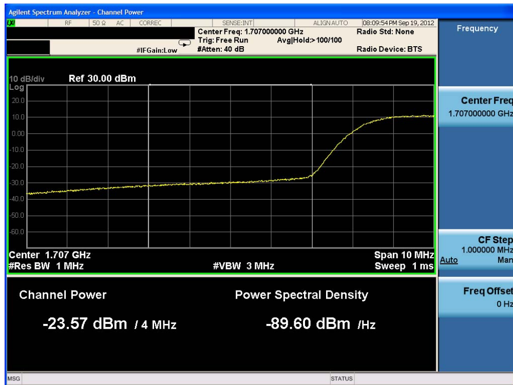
Plot 10-1. Lower Band Edge Plot (QPSK – RB Size 50)
