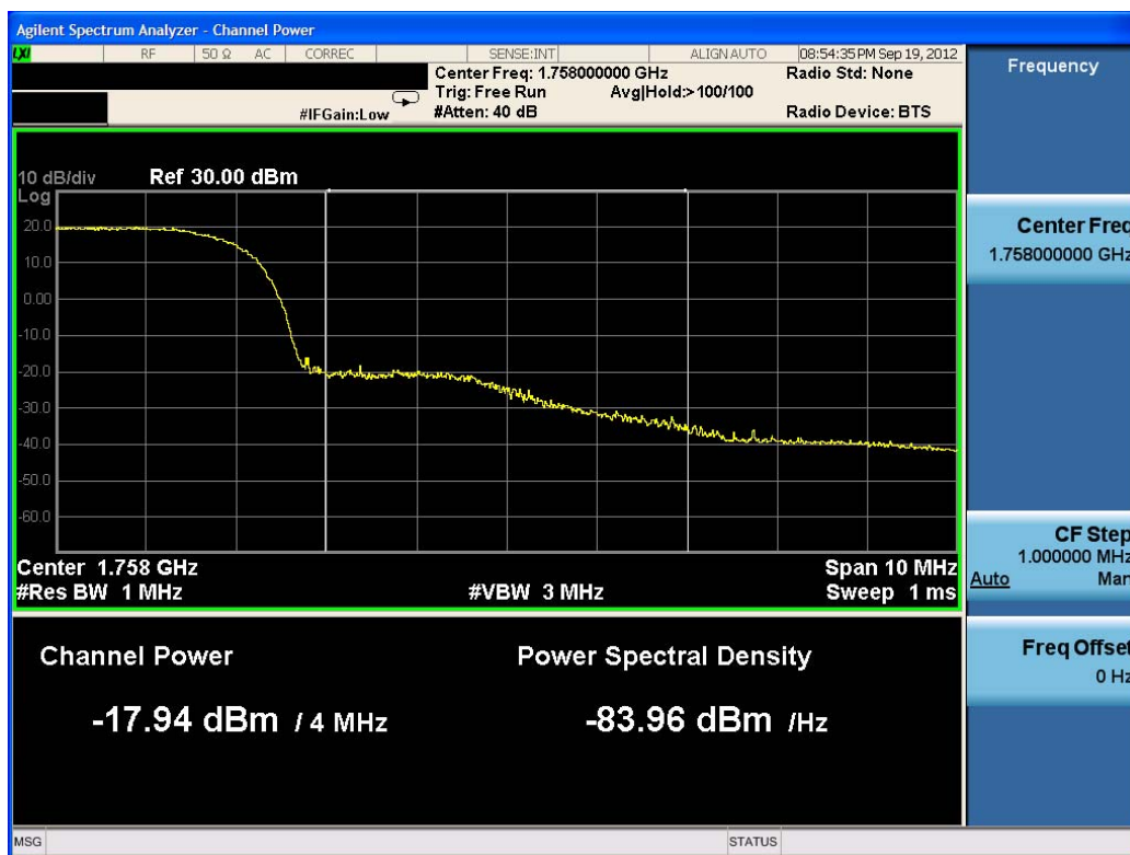
Plot 8-14. Upper Extended Band Edge Plot (QPSK – RB Size 15)
