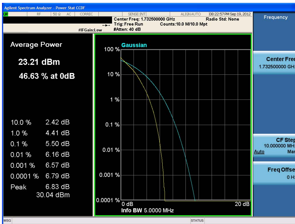
Plot 9-5. Peak to Average Ratio Plot (QPSK - RB Size 25)
