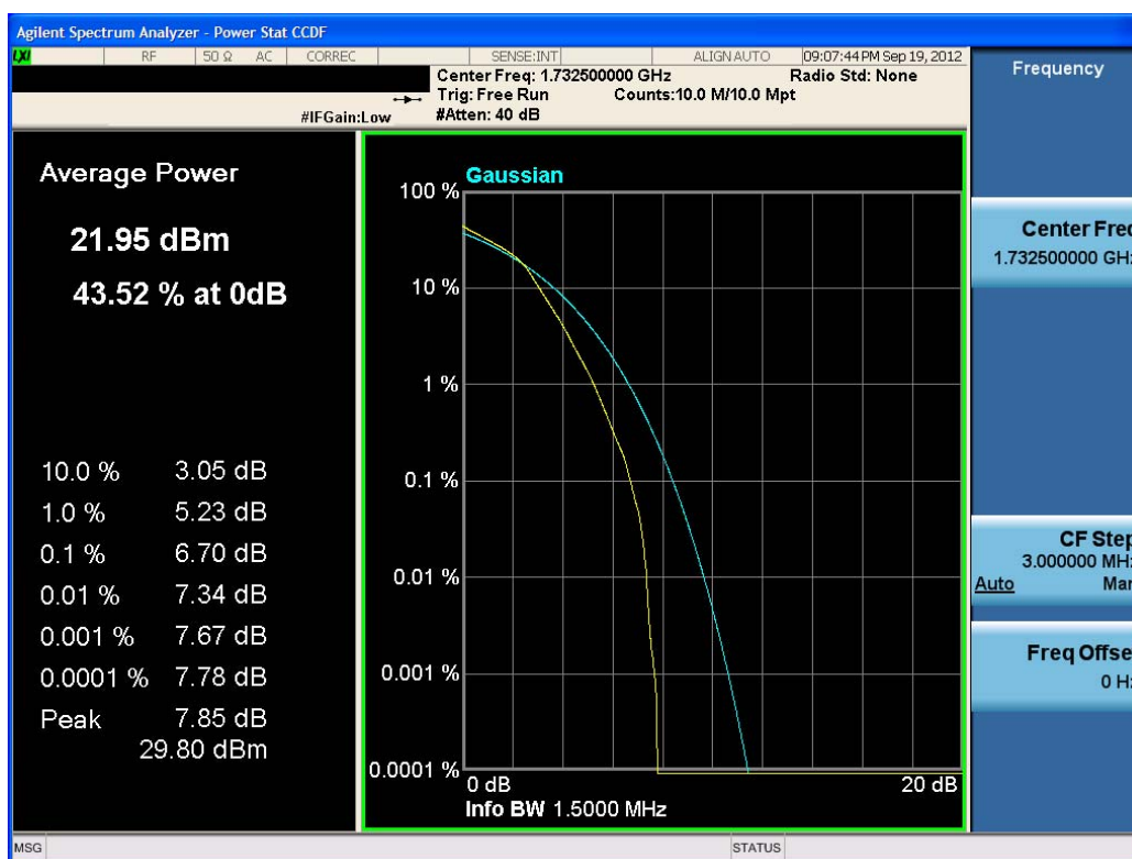
Plot 7-6. Peak to Average Ratio Plot (16QAM - RB Size 6)
