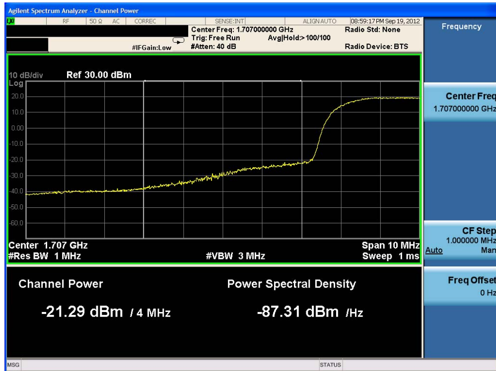
Plot 8-1. Lower Band Edge Plot (QPSK – RB Size 15)
