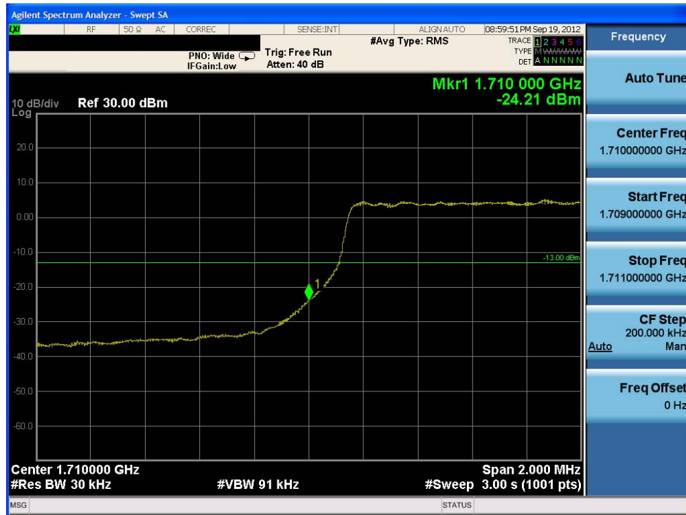
Plot 8-1. Lower Band Edge Plot (QPSK – RB Size 15)
