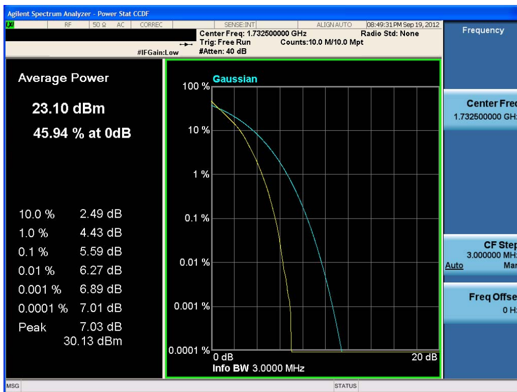
Plot 8-5. Peak to Average Ratio Plot (QPSK - RB Size 15)
