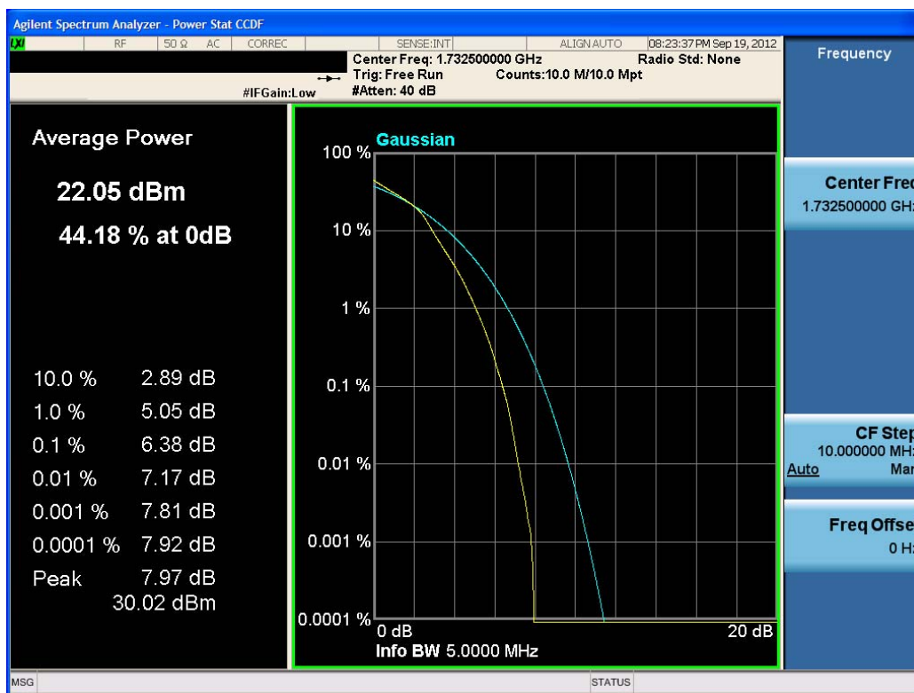
Plot 9-6. Peak to Average Ratio Plot (16QAM - RB Size 25)
