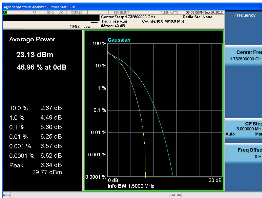
Plot 7-5. Peak to Average Ratio Plot (QPSK - RB Size 6)
