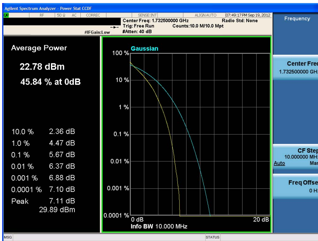
Plot 10-5. Peak to Average Ratio Plot (QPSK - RB Size 50)
