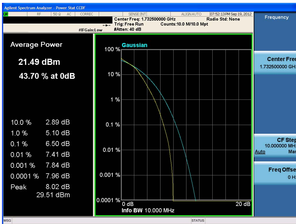
Plot 10-6. Peak to Average Ratio Plot (16QAM - RB Size 50)
