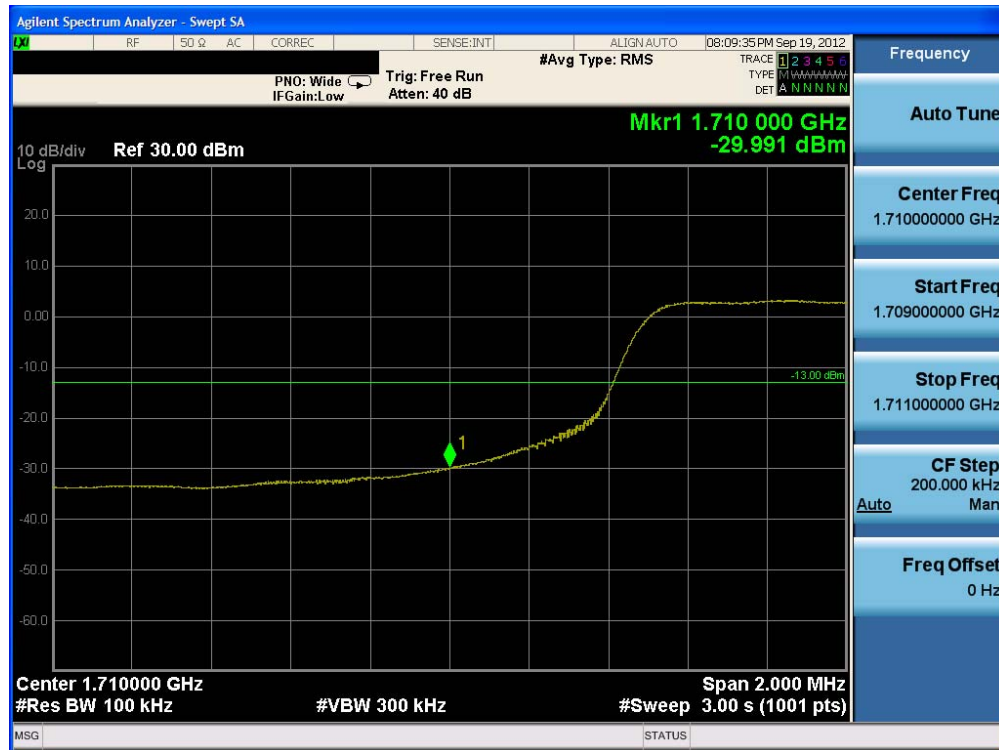
Plot 10-1. Lower Band Edge Plot (QPSK – RB Size 50)
