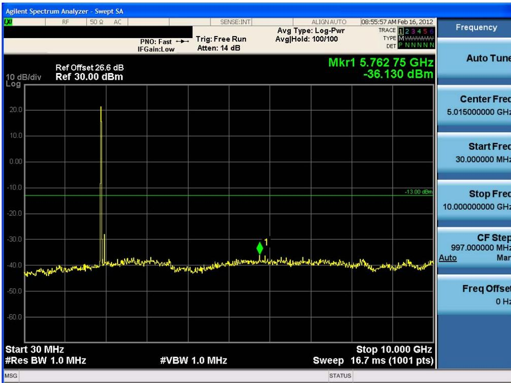
Conducted Spurious Plot (10 MHz BW, QPSK, PCS Band 2 – High Channel)
