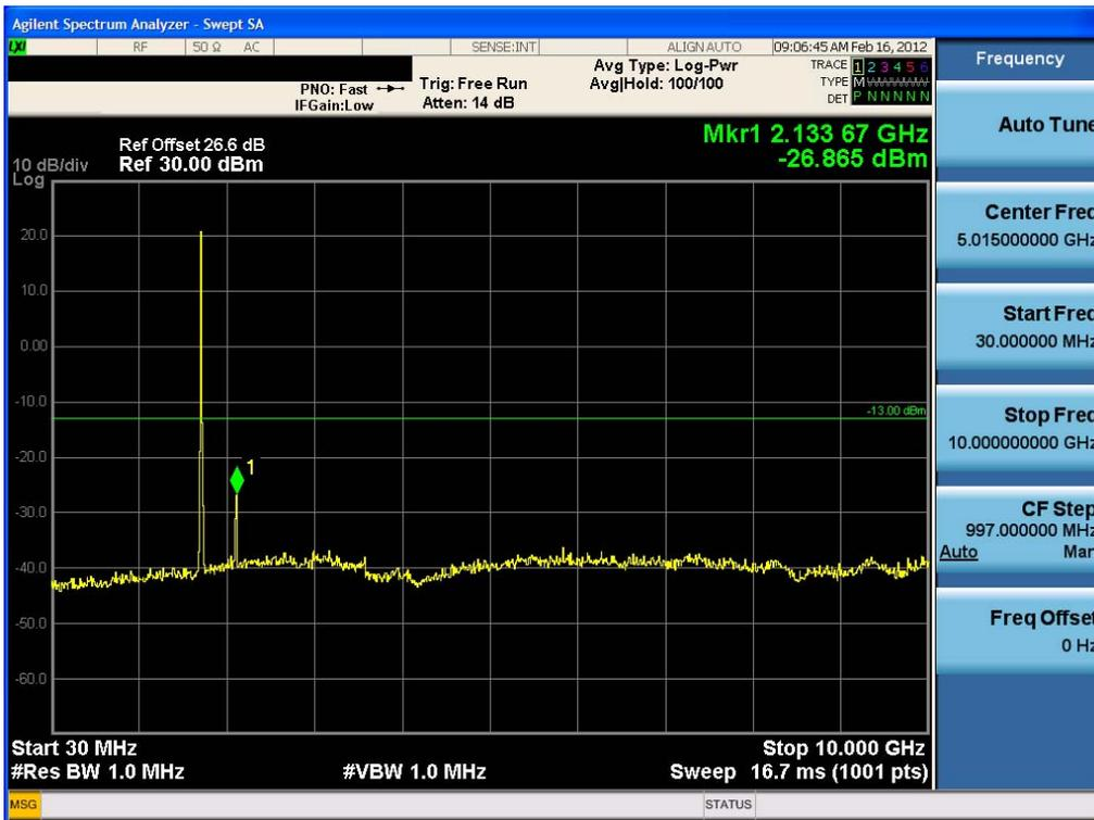
Conducted Spurious Plot (10 MHz BW, QPSK, AWS Band 4 – Mid Channel)
