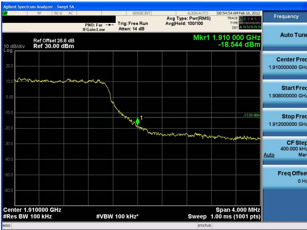
Extended Band Edge Plot (10 MHz BW, QPSK, PCS Band 2 – High Channel)
