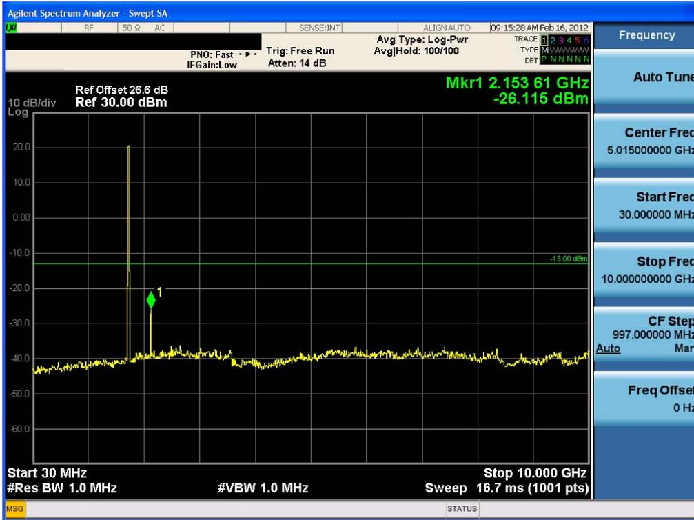
Conducted Spurious Plot (10 MHz BW, QPSK, AWS Band 4 – High Channel)
