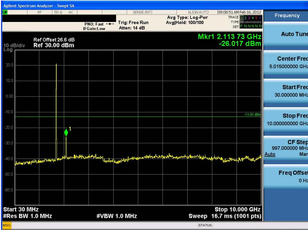
Conducted Spurious Plot (10 MHz BW, QPSK, AWS Band 4 – Low Channel)
