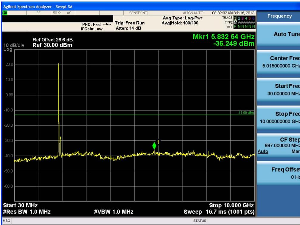
Conducted Spurious Plot (10 MHz BW, QPSK, PCS Band 2 – Mid Channel)
