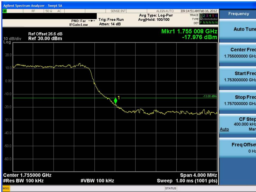
Extended Band Edge Plot (10 MHz BW, QPSK, AWS Band 4 – High Channel)
