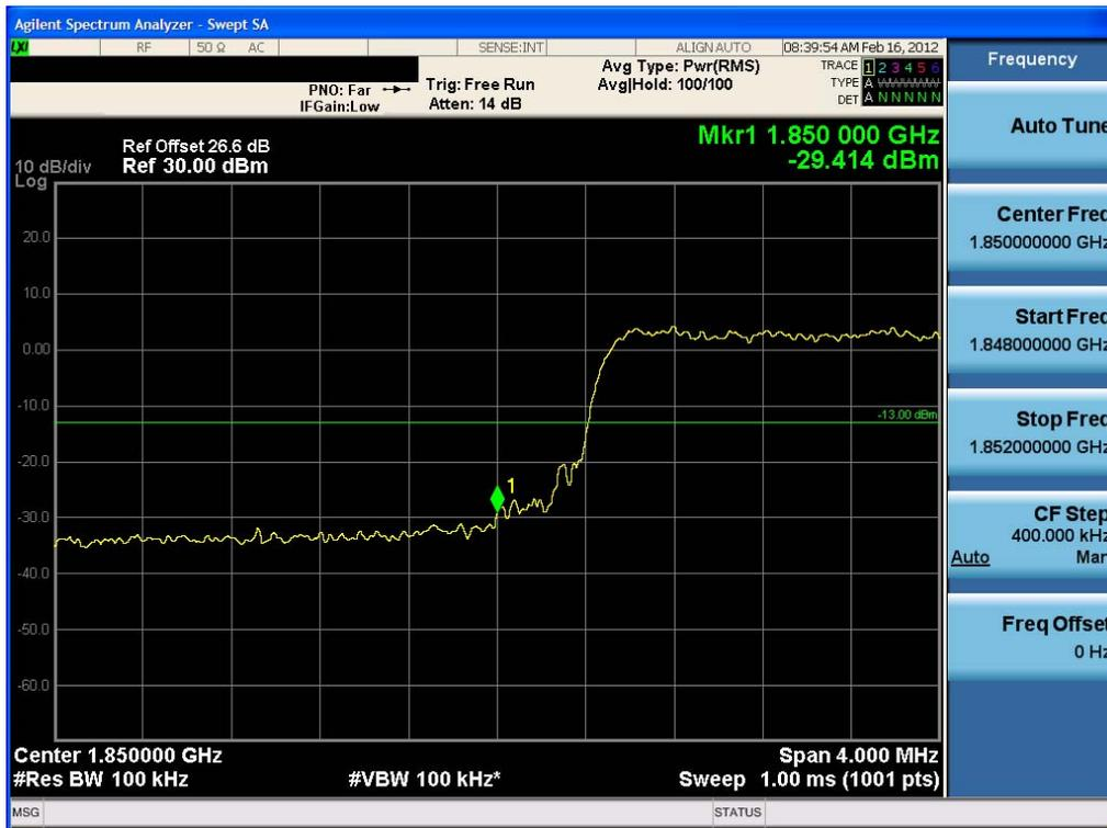
Extended Band Edge Plot (10 MHz BW, QPSK, PCS Band 2 – Low Channel)
