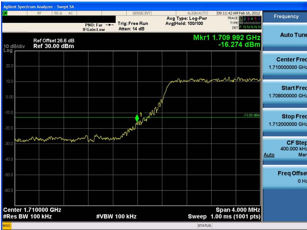
Extended Band Edge Plot (10 MHz BW, QPSK, AWS Band 4 – Low Channel)
