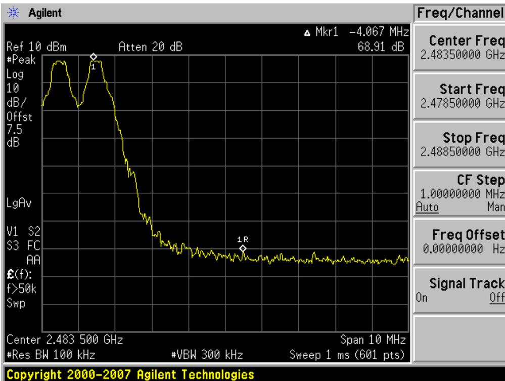
Test Plots with hopping (8DPSK)
