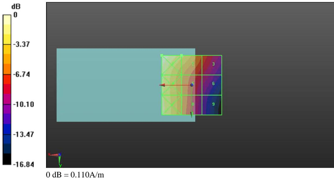
H-field worst-cast test plot for AWS Band
