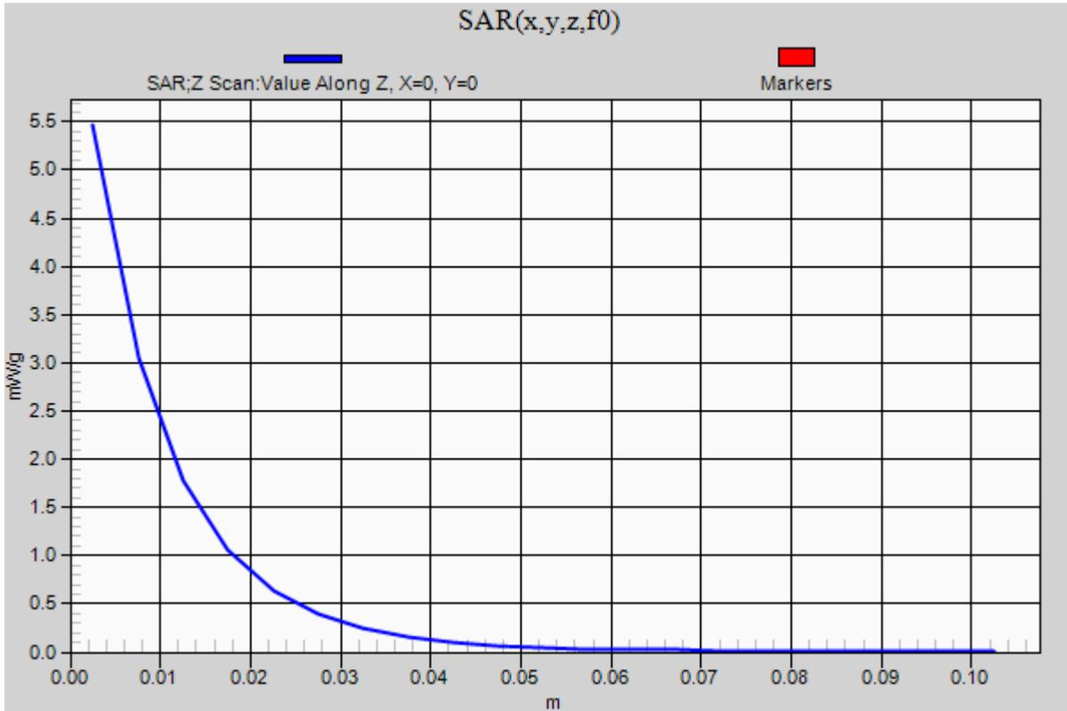
Test Laboratory: UL CCS SAR Lab A
