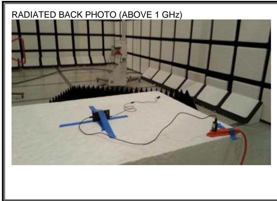
**RADIATED RF MEASUREMENT SETUP FOR PORTABLE CONFIGURATION**
