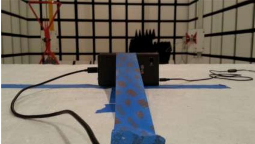
**POWERLINE CONDUCTED EMISSIONS MEASUREMENT SETUP**
