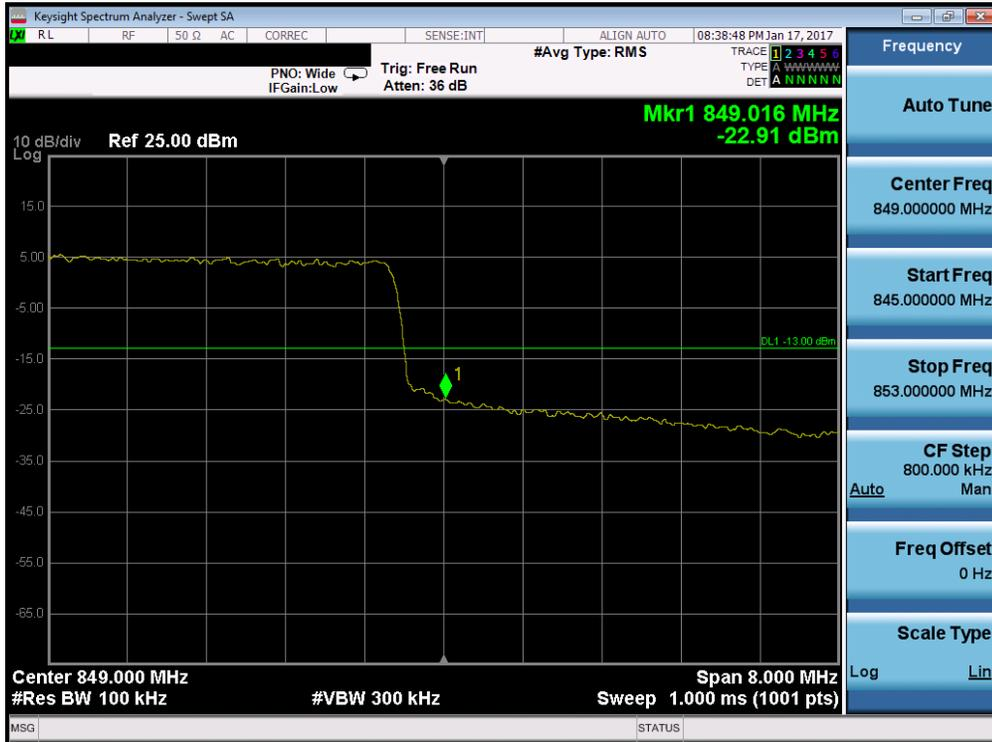
Plot 7-150. Upper Band Edge Plot (Band 5 – 10.0MHz QPSK – RB Size 50)
