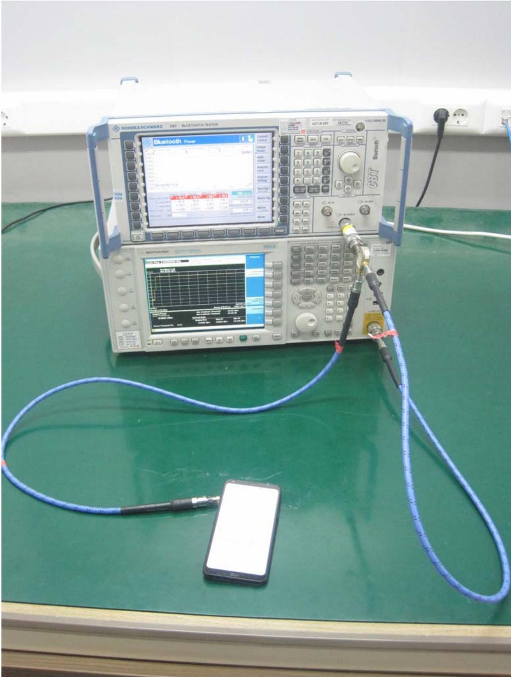
■ Conducted WLAN Test Setup Photo
