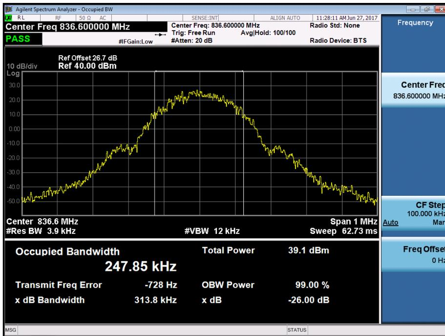
■ GSM850 MODE (251 CH.) Occupied Bandwidth
