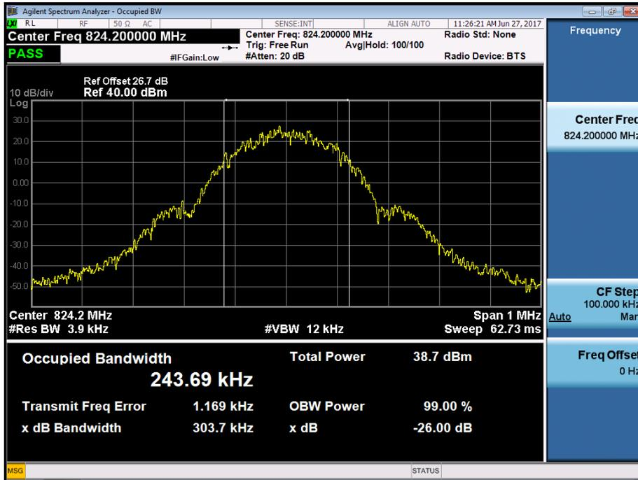
■ GSM850 MODE (190 CH.) Occupied Bandwidth
