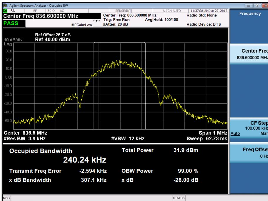
■ GSM1900 MODE (512 CH.) Occupied Bandwidth
