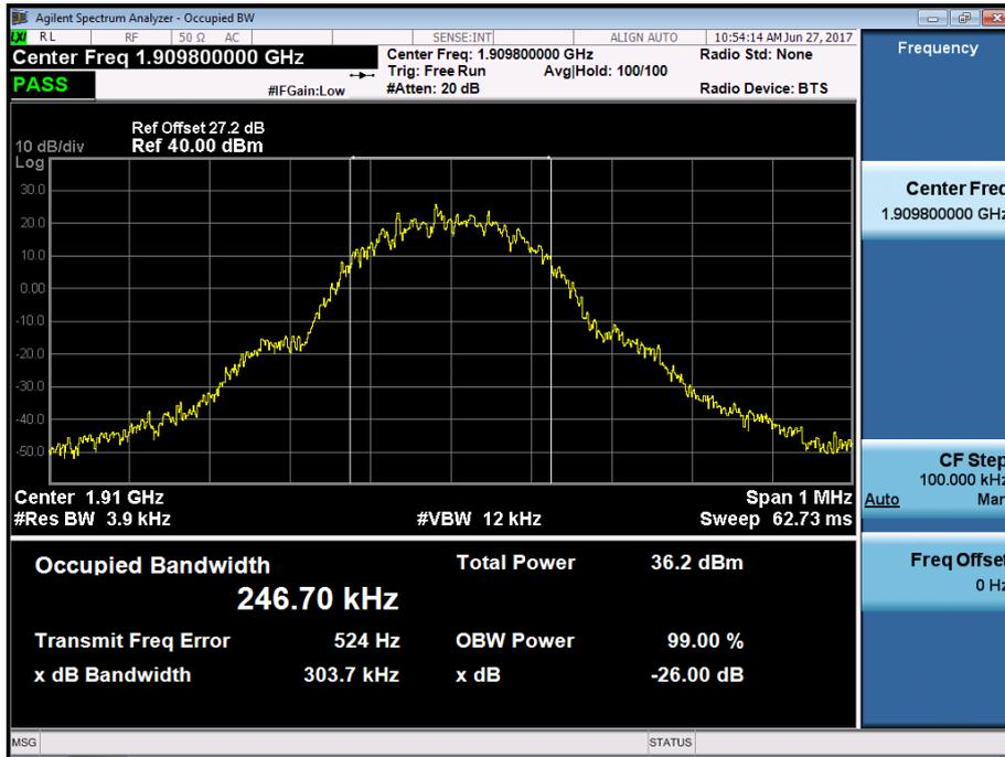
■ GSM1900 EDGE (810 CH.) Occupied Bandwidth
