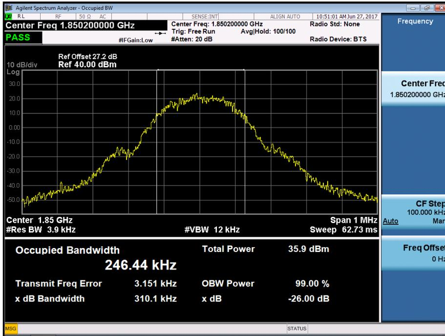
■ GSM1900 MODE (661 CH.) Occupied Bandwidth
