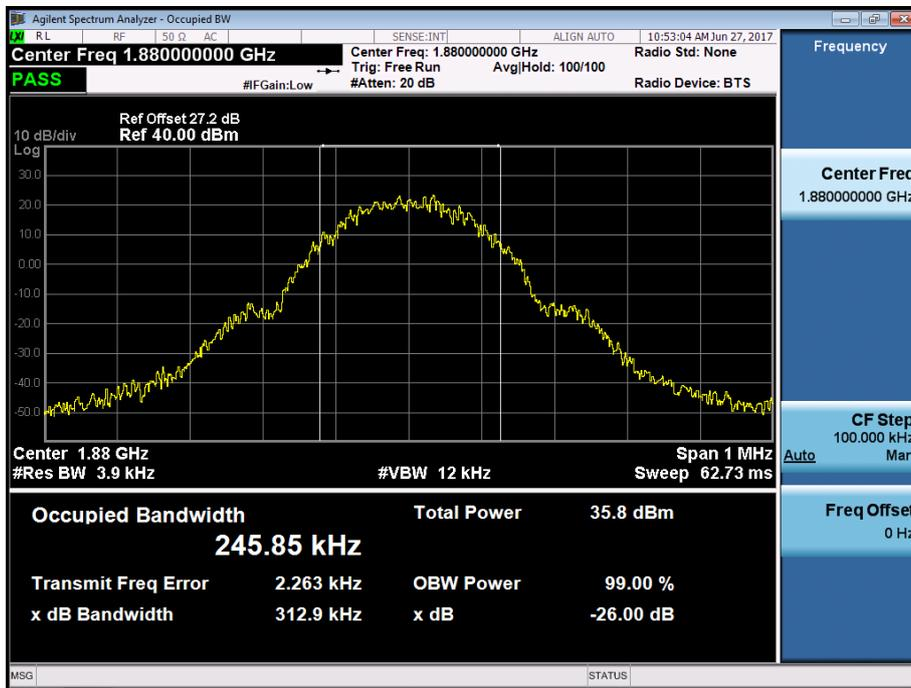
■ GSM1900 MODE (810 CH.) Occupied Bandwidth
