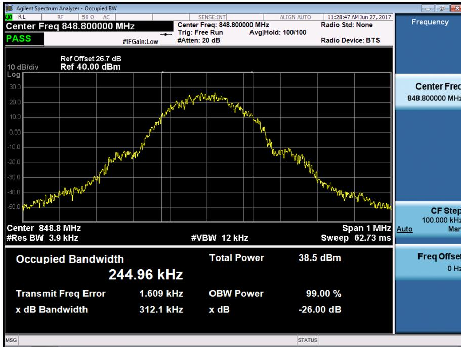
■ GSM850 EDGE (190 CH.) Occupied Bandwidth
