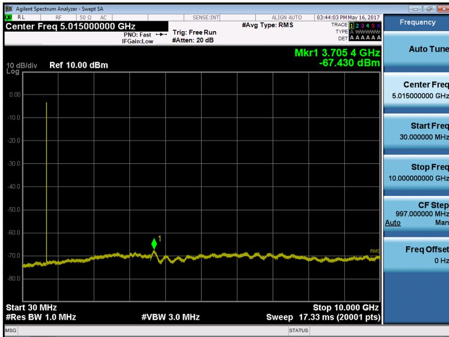
BAND 17. Conducted Spurious Plot\_ (23790ch\_10MHz\_QPSK\_RB 1\_0)
