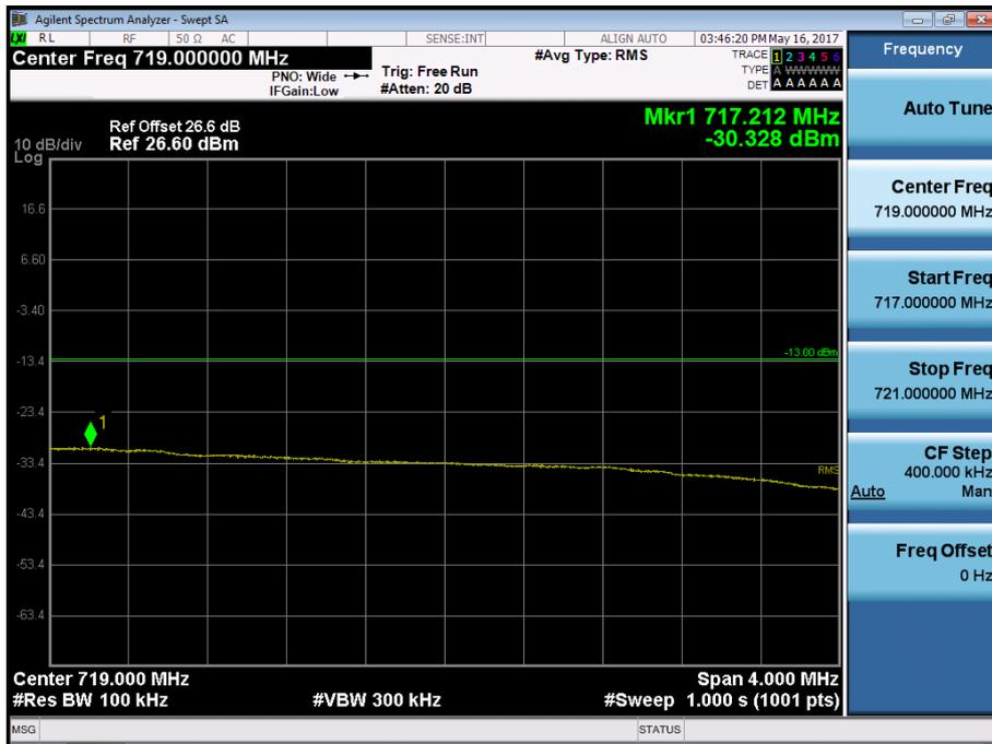
BAND 17. Conducted Spurious Plot\_ (23755ch\_5MHz\_QPSK\_RB 1\_0)
