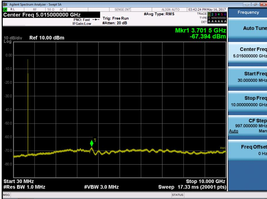
BAND 17. Conducted Spurious Plot\_ (23780ch\_10MHz\_QPSK\_RB 1\_0)
