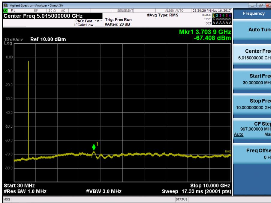
BAND 17. Conducted Spurious Plot\_ (23790ch\_5MHz\_QPSK\_RB 1\_0)
