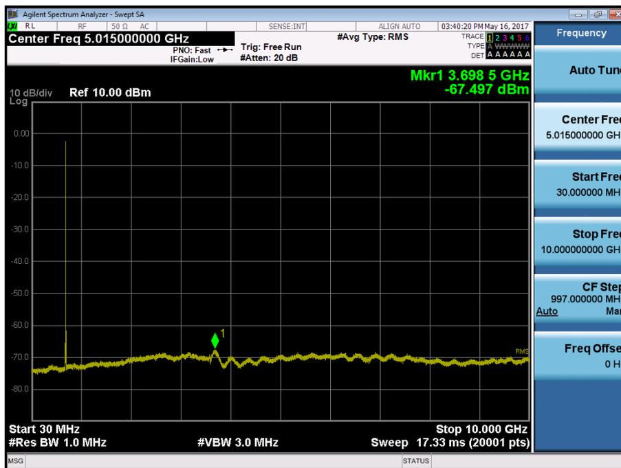
BAND 17. Conducted Spurious Plot\_ (23825ch\_5MHz\_QPSK\_RB 1\_0)
