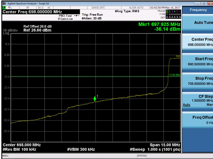
BAND 17. Lower Extended Band Edge Plot (10M BW Ch.23780 QPSK\_RB50\_0) -3
