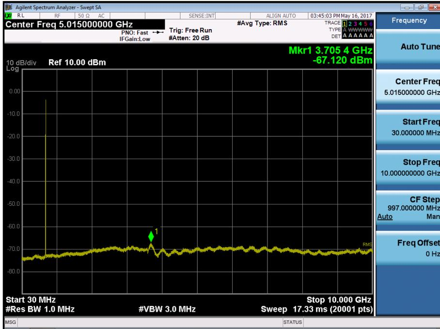
BAND 17. Conducted Spurious Plot\_ (23800ch\_10MHz\_QPSK\_RB 1\_0)
