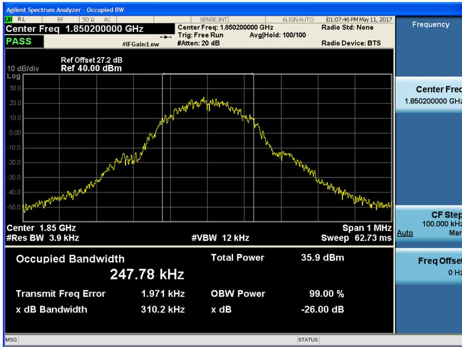
■ GSM1900 MODE (661 CH.) Occupied Bandwidth
