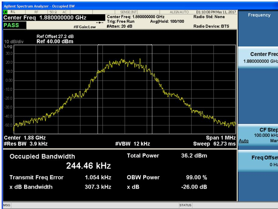
■ GSM1900 MODE (810 CH.) Occupied Bandwidth
