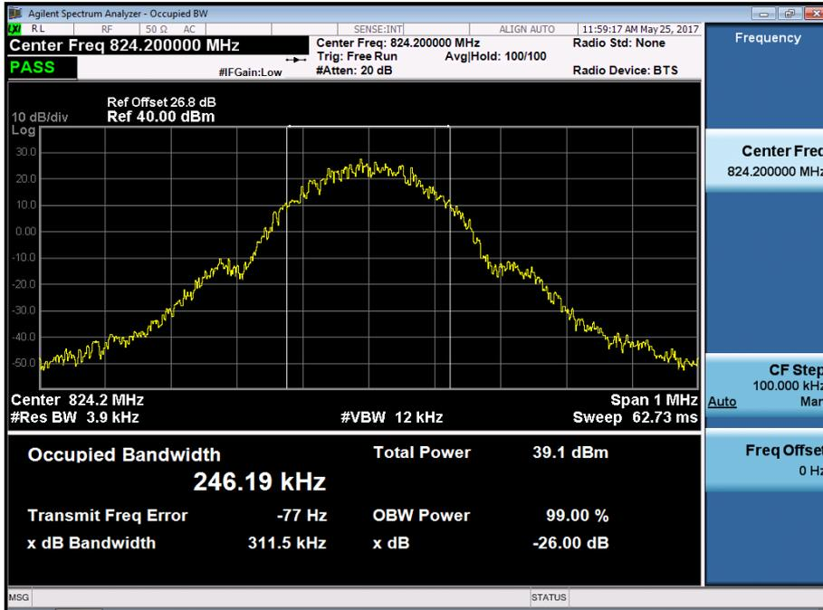
■ GSM850 MODE (190 CH.) Occupied Bandwidth
