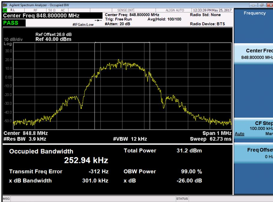
■ GSM1900 MODE (512 CH.) Occupied Bandwidth
