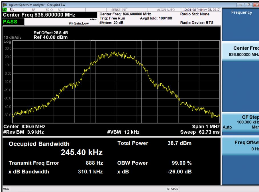
■ GSM850 MODE (251 CH.) Occupied Bandwidth
