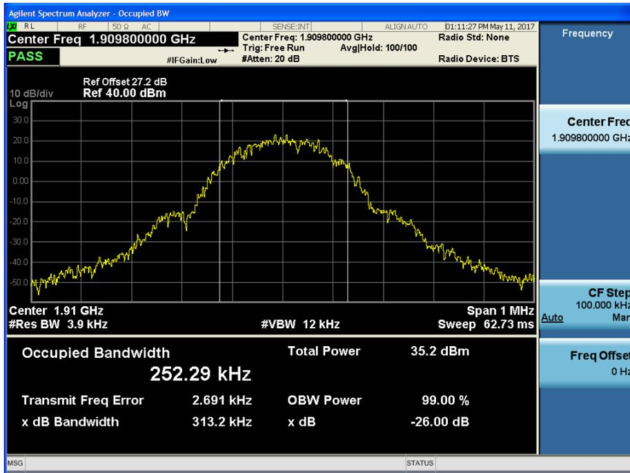
■ GSM1900 EDGE (810 CH.) Occupied Bandwidth
