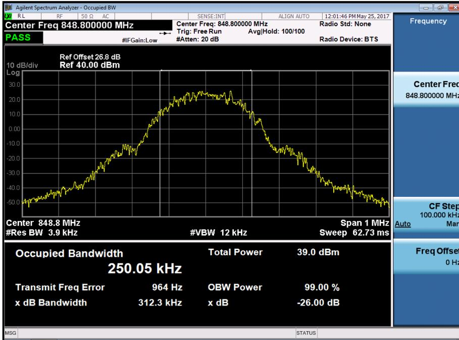
■ GSM850 EDGE (251 CH.) Occupied Bandwidth
