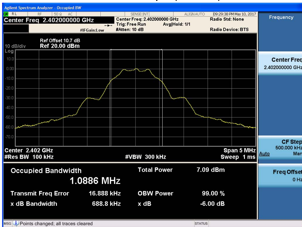
6 dB Bandwidth plot (Low-CH 0)
