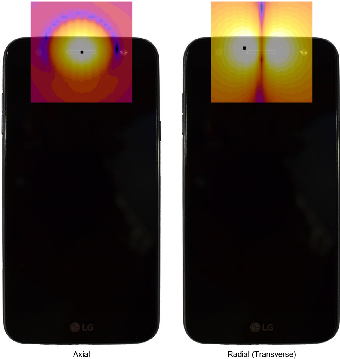
Axial Radial (Transverse) Figure 13-3 T-Coil Scan Overlay Magnetic Field Distributions
