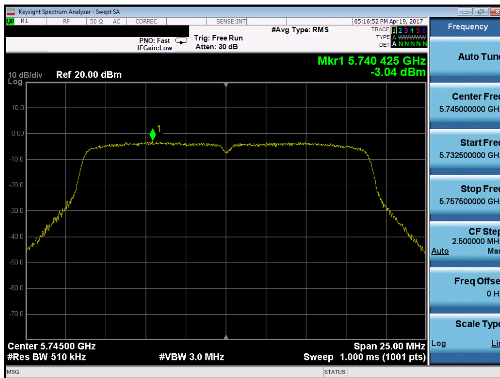
Plot 7-62. Power Spectral Density Plot (20MHz BW 802.11n (UNII Band 3) – Ch. 149)
