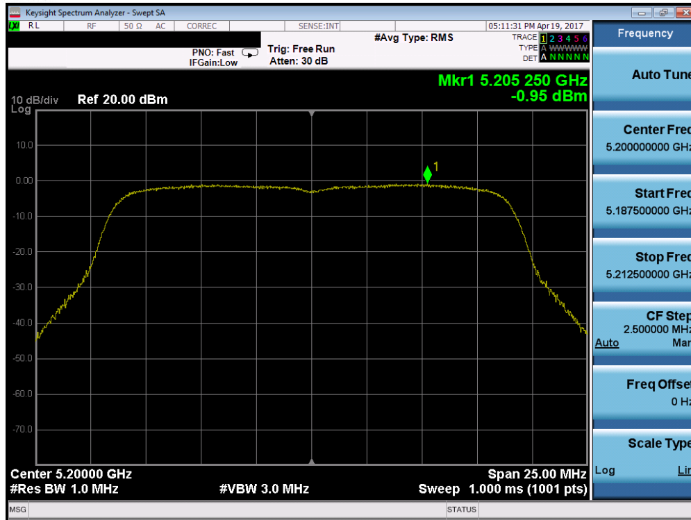
Plot 7-38. Power Spectral Density Plot (20MHz BW 802.11n (UNII Band 1) – Ch. 40)
