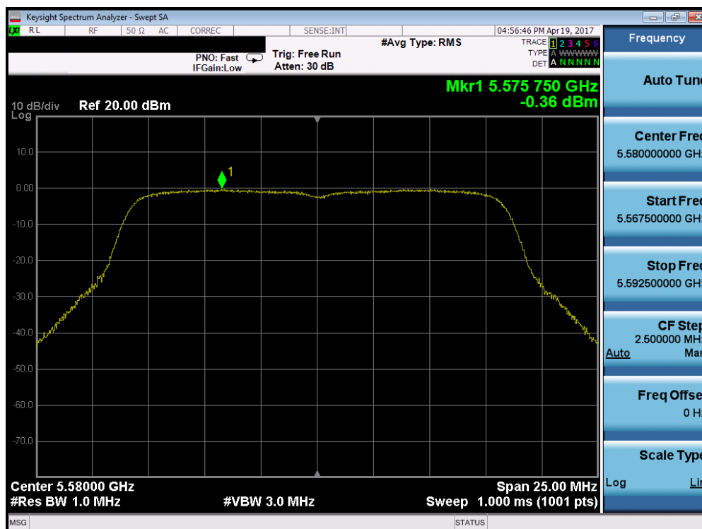
Plot 7-51. Power Spectral Density Plot (802.11a (UNII Band 2C) – Ch. 116)
