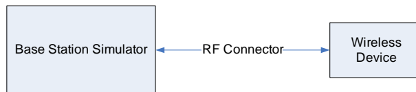
Figure 9-3 Power Measurement Setup
