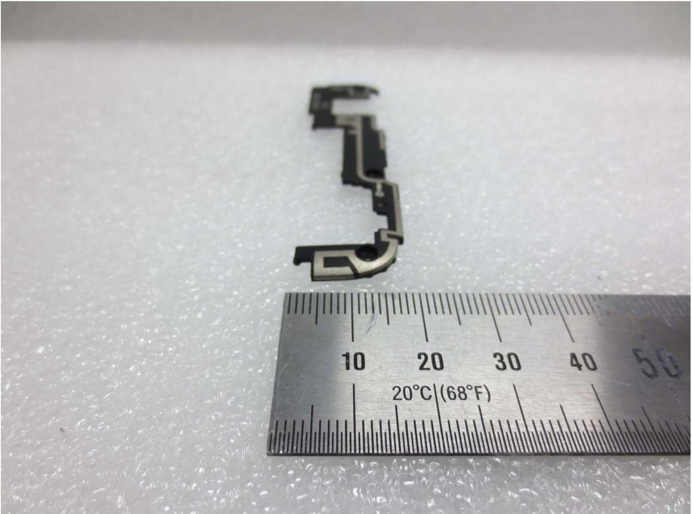
■ BT & WLAN Antenna INTERNAL PHOTO
