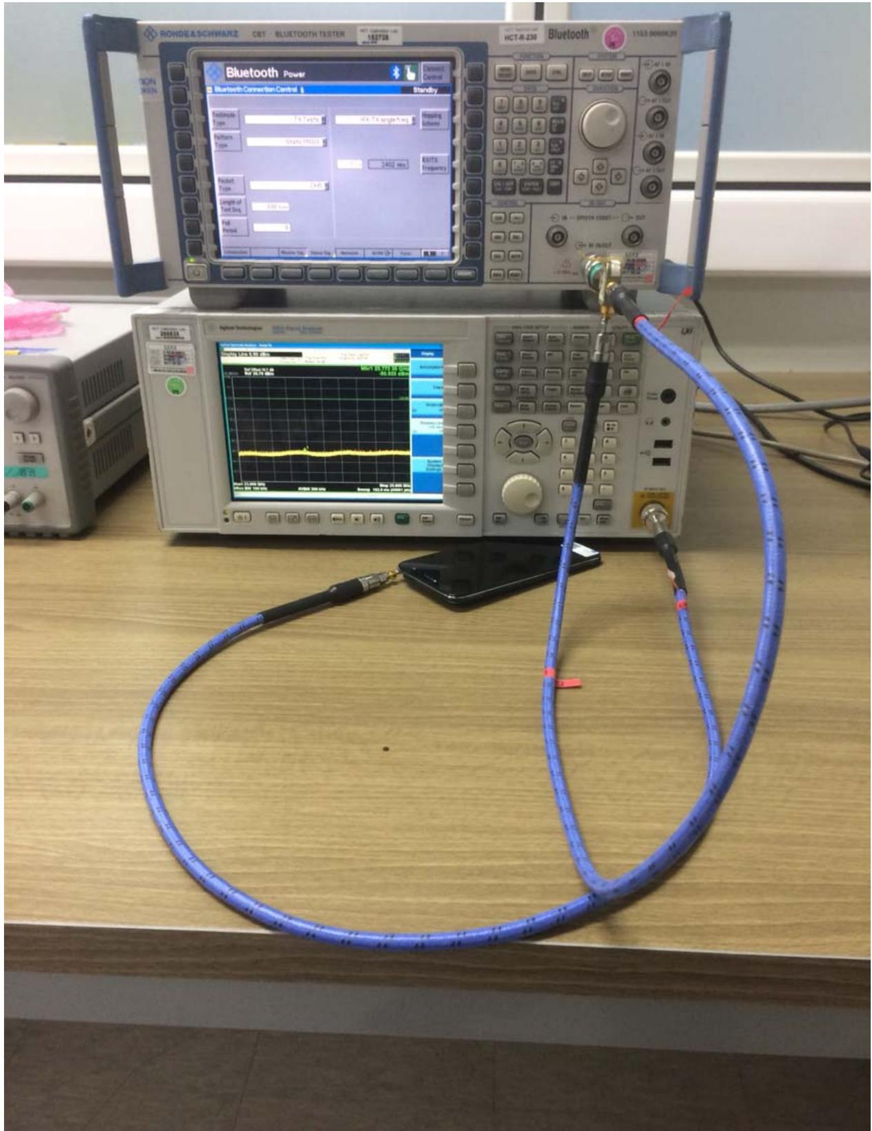
■ Conducted WLAN Test Setup Photo
