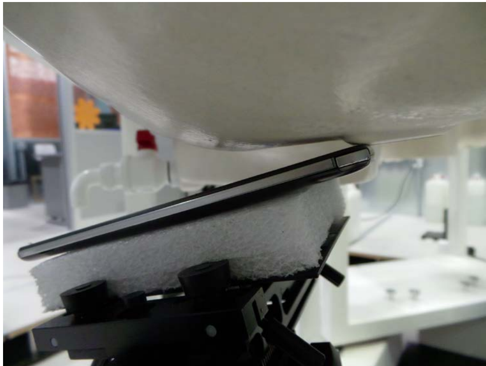
SAR Test Setup Photo 4: Left Tilt
