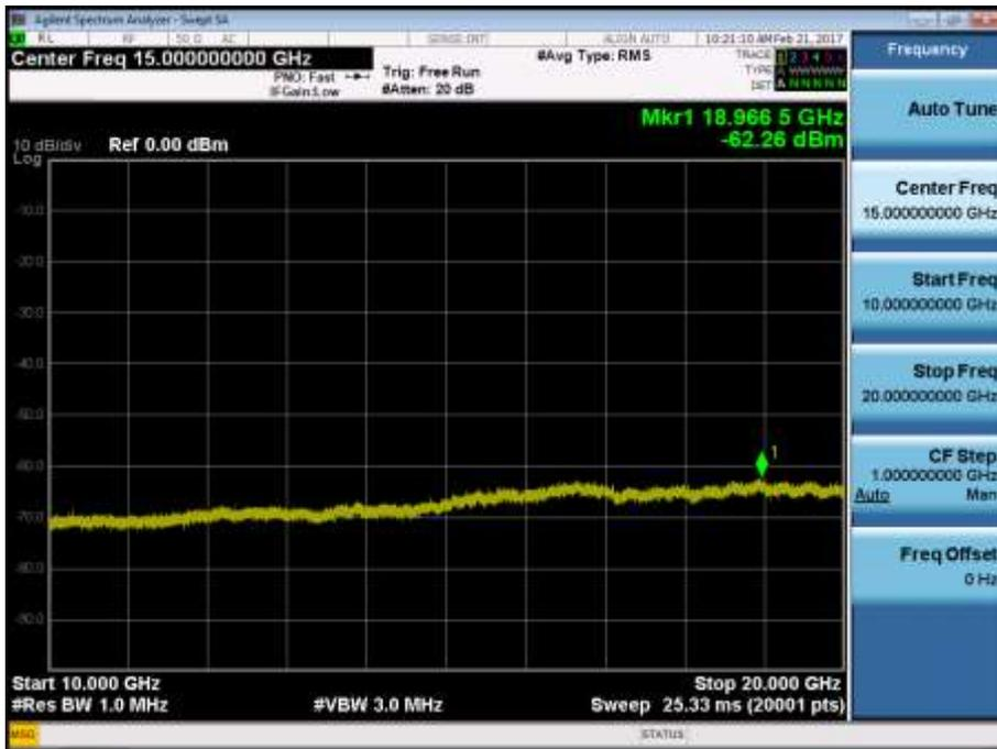
BAND 2. Conducted Spurious\_1 (18900ch\_10MHz\_QPSK\_RB 1\_0)
