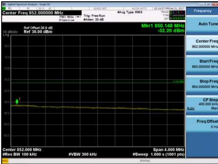
BAND 2. Conducted Spurious\_1 (18607ch\_1.4MHz\_QPSK\_RB 1\_0)
