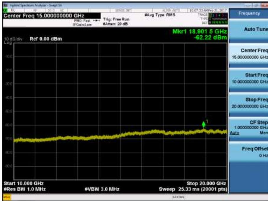
BAND 2. Conducted Spurious\_1 (18900ch\_3MHz\_QPSK\_RB 1\_0)
