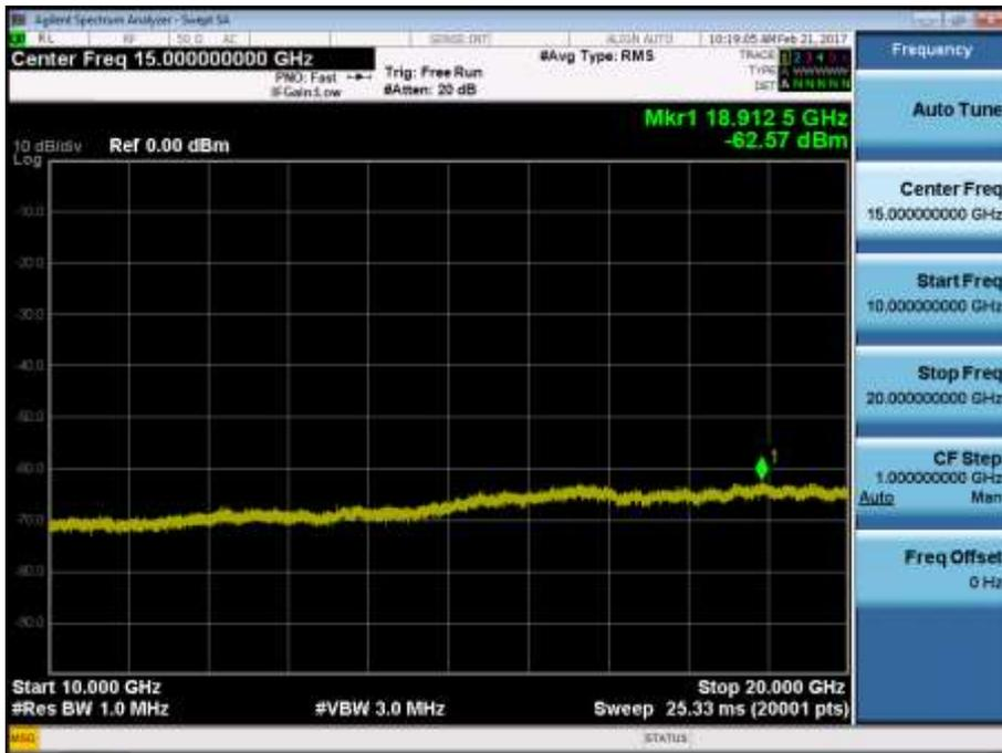
BAND 2. Conducted Spurious\_1 (18650ch\_10MHz\_QPSK\_RB 1\_0)
