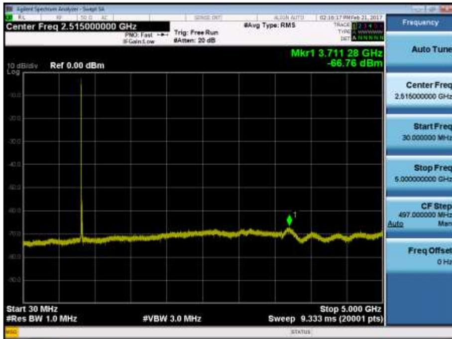
BAND 5. Conducted Spurious Plot \_2 (20525ch\_10MHz\_QPSK\_RB 1\_0)
