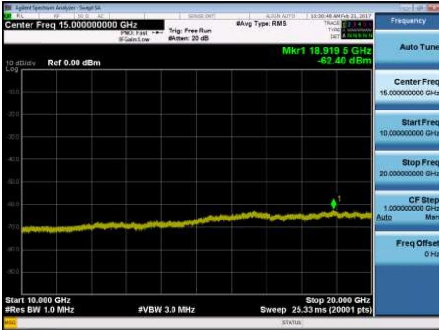
BAND 2. Conducted Spurious\_1 (18700ch\_20MHz\_QPSK\_RB 1\_0)
