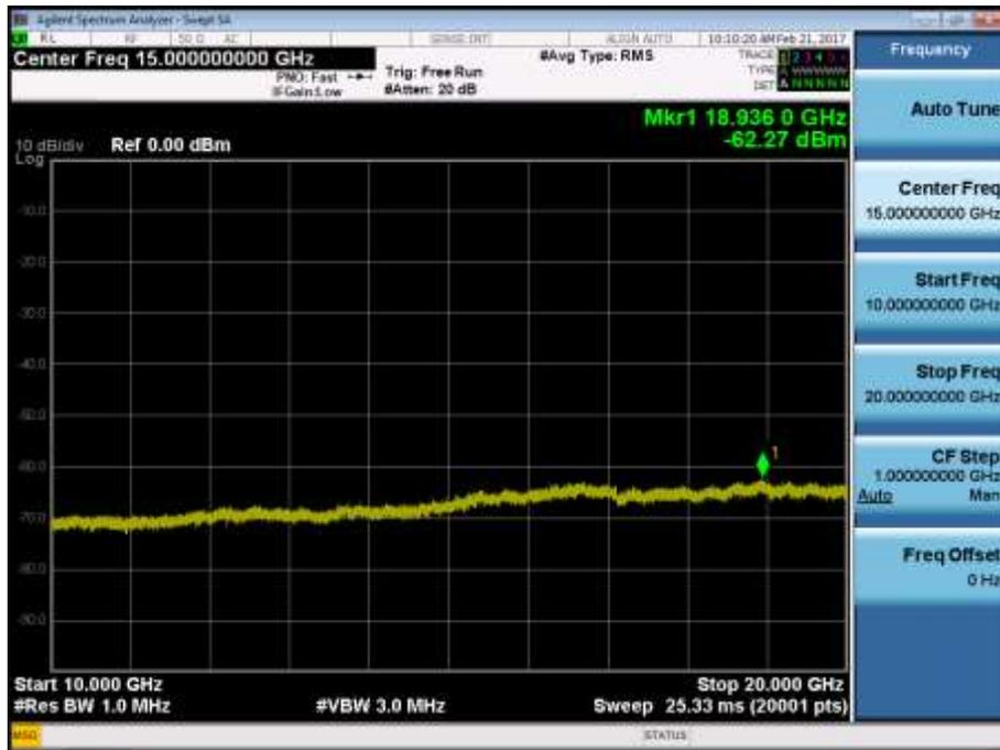
BAND 2. Conducted Spurious\_1 (19185ch\_3MHz\_QPSK\_RB 1\_0)
