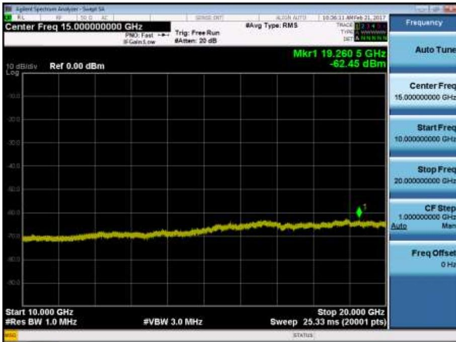
BAND 2. Conducted Spurious\_1 (19100ch\_20MHz\_QPSK\_RB 1\_0)
