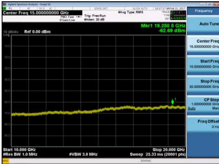
BAND 2. Conducted Spurious\_1 (19175ch\_5MHz\_QPSK\_RB 1\_0)
