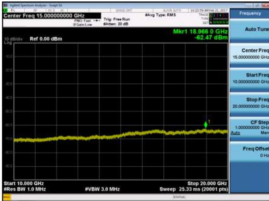
BAND 2. Conducted Spurious\_1 (19150ch\_10MHz\_QPSK\_RB 1\_0)
