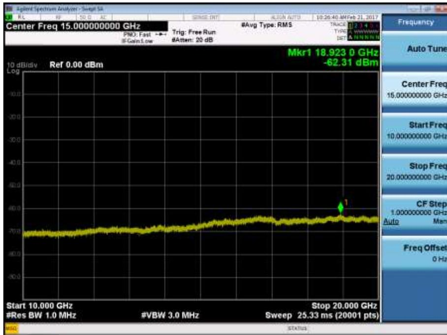
BAND 2. Conducted Spurious\_1 (18900ch\_15MHz\_QPSK\_RB 1\_0)
