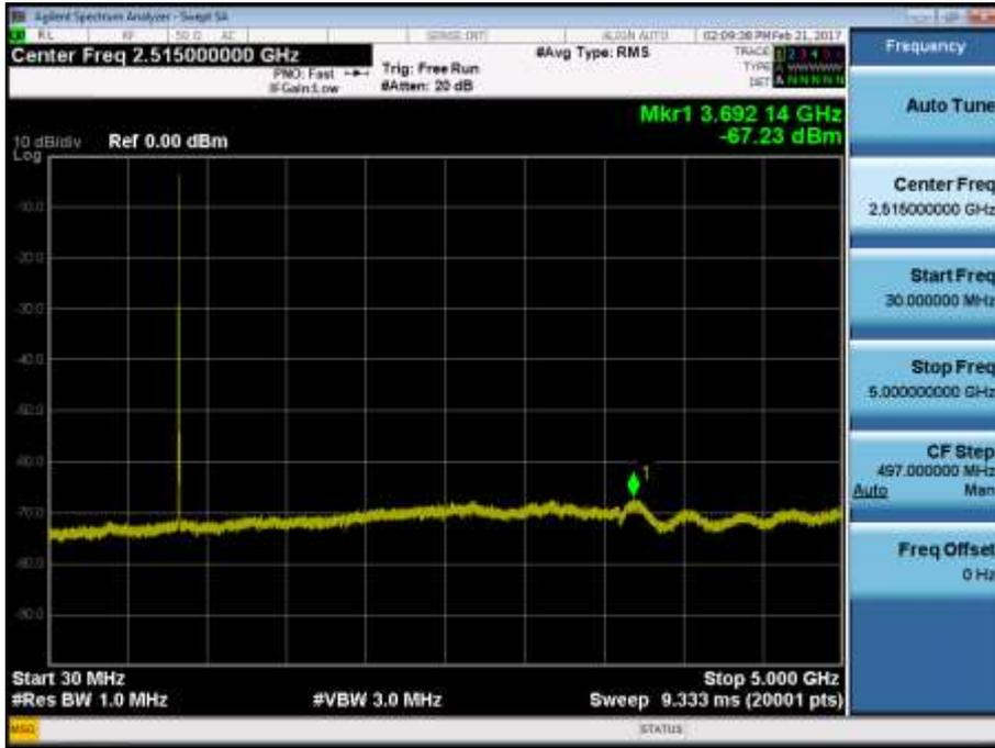
BAND 5. Conducted Spurious Plot \_2 (20635ch\_3MHz\_QPSK\_RB 1\_0)
